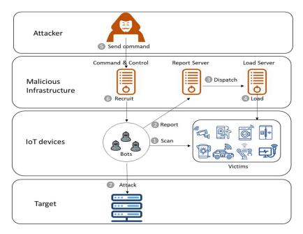
Figure 4. A flow diagram of an IoT botnet.
