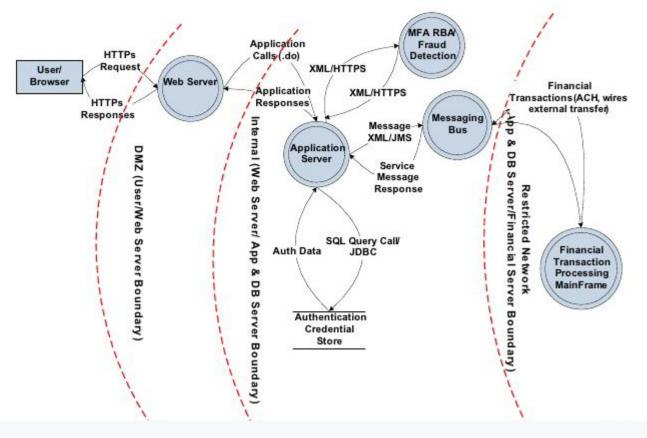
https://threatmodeler.com/data-flowdiagrams-process-flow-diagrams/ System engineers developed data flow diagrams to provide a high-level visualization of how an application works within a system to move, store and manipulate data. The intended use of DFDs was to provide engineers a way of efficiently communicating their structured system analysis. Security professionals added the concept of trust boundaries to DFDs in the early 2000s to make them more applicable for threat modeling.
