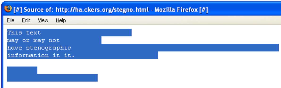
Fig 16.6 – Spaces, tabs and newlines placed within a small HTML file - highlighted to be more visible
