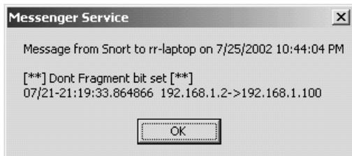
**Figure 4-2** SMB alert display window.
