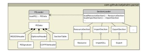
Figure 4.3: Structure of PortEx' PE format parser
