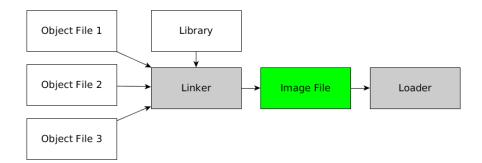
Figure 3.1: The linker combines object files and libraries to an image file, which is used as input by the loader
