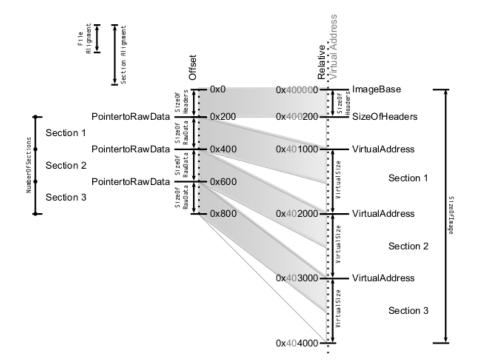
Figure 3.5: Mapping a PE file from disk (left side) to memory (right side) by [Alb13].
