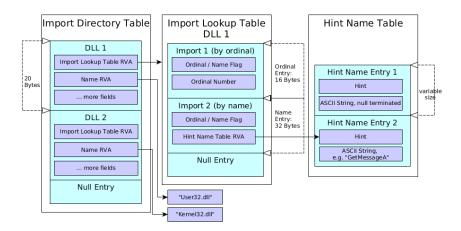
Figure 3.4: Typical Import Section layout
