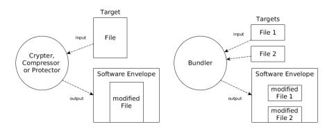
Figure 2.6: Functionality of packers
