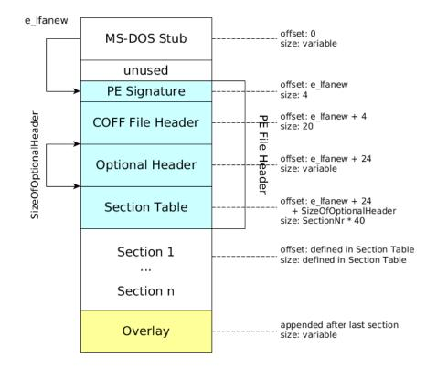
Figure 3.2: Structure of a PE file
