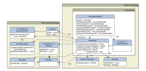
Figure 4.10: Visualiser package structure and dependencies
