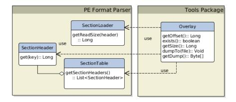
Figure 4.9: Overlay tool structure and dependencies
