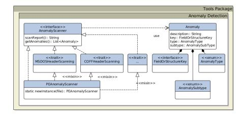
Figure 4.8: Anomaly detection package structure
