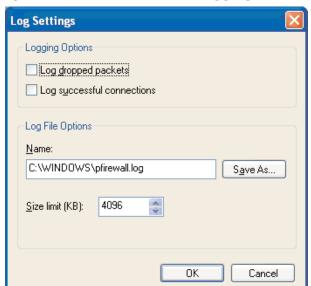
Figure 5.6 Configure Windows XP Firewall Logging
