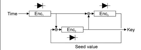
Relies on strength of triple DES encryption and supplied encryption key
