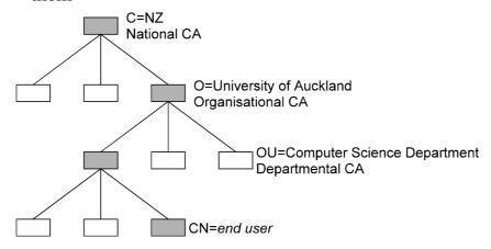
Top-level CA is called the root CA, aka "the single point of failure"
