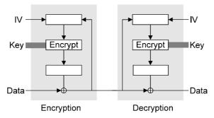
This converts a block cipher to a stream cipher (with the accompanying vulnerabilities)
