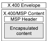
X.400 security required using (and trusting) X.400 MTA; MSP requires only trusted endpoints
