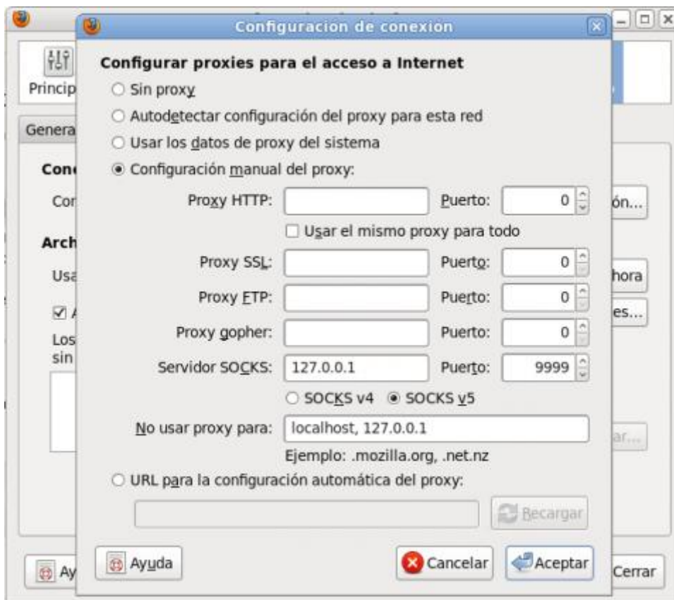
Figura 4.1: Firefox Proxy (SOCKS) configuration
