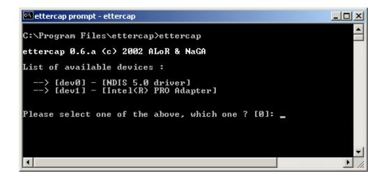
4. Once this is done, a quick ARP scan is preformed in order to map out the network, and then the following screen is shown:
