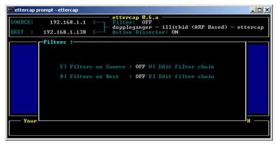
6. To activate the filter we need to press "S", and then we should see the filter status turn to "ON".
