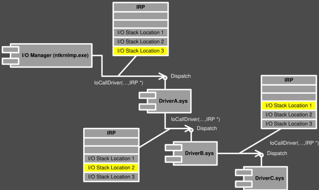
Each I/O Request Packet (IRP) contains a stack at the end of its structure to keep track of the current device driver in the device driver stack. It is implemented similarly to a thread stack: its pointer (slot index) is decremented from bottom to top.
