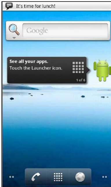
Figure 44. The notification, right as it is being added, showing the "ticker text"
