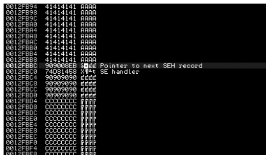
Figure 15-4: Quick TFTP's initial SEH overwrite
