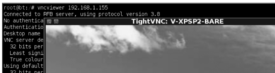
Figure 4-18: Connecting to VNC with no authentication using vncviewer
