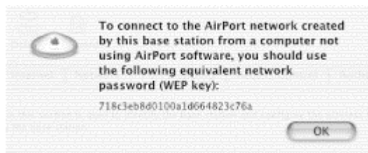
Figure B-13. Printing out the WEP key in hexadecimal for use by non-Apple 802.11 stations
