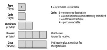
The Type field is set to one, which is the value for the Destination Unreachable message. The Code field supplies more information about the reason why the datagram was not delivered. The possible codes are listed in <u>Table 4-3</u>. The data portion of the ICMP message contains parts of the original message—as much as will fit into the ICMP message.
