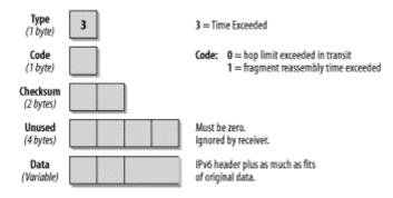
The Type field carries the value 3, specifying the Time Exceeded message. The Code field can be set to 0, which means hop limit exceeded in transit, or to 1, which means that the fragment reassembly time is exceeded. The data portion of the ICMP message contains parts of the original message—as much as fits into the ICMP message, depending on the MTU used.
