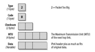
The Type field has the value 2, which identifies the Packet Too Big message. In this case, the Code field is not used and is set to zero. The important information for this type of message is the MTU field, which contains the MTU size of the next hop link.
