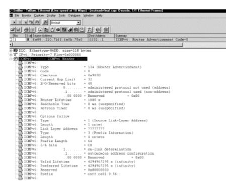
The router sends the advertisement to the all-nodes multicast address ff02::1, so all nodes on the link receive it. Looking at this packet in the detail window, we can see how the router is configured. The hop limit is set to 32. DHCP (administered protocol) is not used for address information, but is used by the
