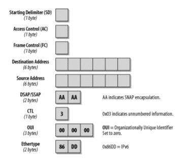
The first three fields for Starting Delimiter (SD), Access Control (AC), and Frame Control (FC) each have a size of 1 byte. The fields for Source and Destination Address each have 6 bytes. The DSAP and SSAP fields are set to the value AA, which indicates SNAP encapsulation. The Control field (CTL) is set to the
