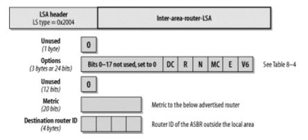
In the tree-building process, this LSA represents an informational pointer associated with the ABR for attaching an ASBR to the SPF tree.
