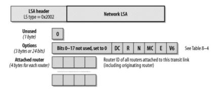
The Options field is set to the logical OR of the Options field received from the Link-LSA of all the routers attached to this transit link. (See <u>Section 8.2.5.9.</u>) This provides the common optional capabilities supported by all routers on this link.
