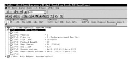
This trace file shows all of the header fields I have discussed and how they are presented in a trace file. The Version field is set to 6 for IPv6. The Priority and the Flow Label fields are not used in this packet and are set to zero. The Payload Length is 40 and the Next Header value is set to 58 for ICMPv6. The Hop Limit is set to 128 and the Source and Destination addresses contain the link local addresses of my IPv6 nodes.
