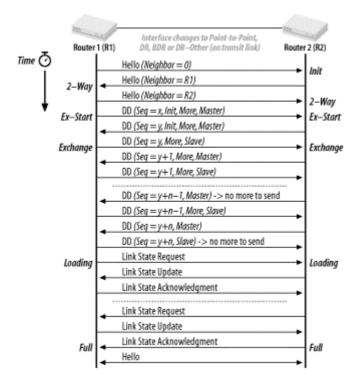
The two routers forming an adjacency start communicating the contents of their LSDB. This phase is called the database description exchange. Once the routers know the contents of each other's databases, they request the missing or outdated information. This is the loading phase. After completing the loading phase, the routers are fully adjacent. Continuous sending of Hello packets prevents the adjacency from timing out.
