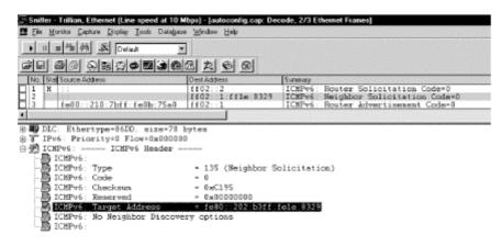
The address is still in the tentative state, so the source address in the IPv6 header is the unspecified address again. The solicitation is sent out to the solicited-node multicast address. The important field here is the target address in the ICMPv6 header, which is highlighted. If a node already uses this address, it will already be a member of this solicited-node multicast address group and will reply with a Neighbor Advertisement. Then the autoconfiguration process will stop.
