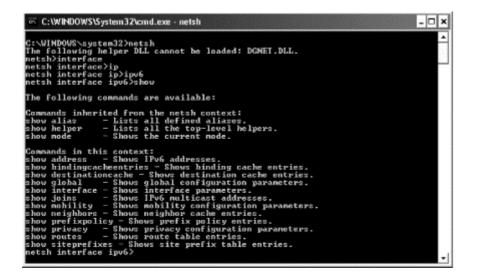
From the command prompt, I entered *netsh* to start the utility. Then I started to change to the context where I can work with my IPv6 configuration. First, I changed to the context *interface*, then to the context *ip*, and finally to the context *ipv6*. The command *show* always returns a list of the commands that are available in the context where I use it.
