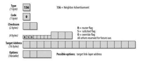
The type of address in the IP header indicates whether the message is the answer to a solicitation or an unsolicited message. In case of a solicited advertisement, the destination IP address is the source address of the interface that sent the solicitation. If the message is the reply to a DAD message that originated from an unspecified source address, the reply will go to the all-nodes multicast address of FF02:1. The same is true for all unsolicited periodic advertisements.
