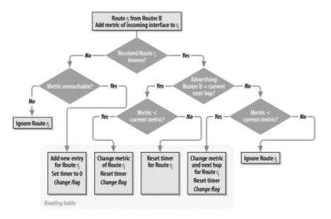
Router A receives a routing update from router B and has already added the distance of 1 to each route  $r_i$  advertised by B. For each route  $r_i$ , the router steps through the algorithm depicted in Figure 8-2. According to Figure 8-2, the routing table will be updated if the following criteria are true; otherwise, route  $r_i$  is discarded:
