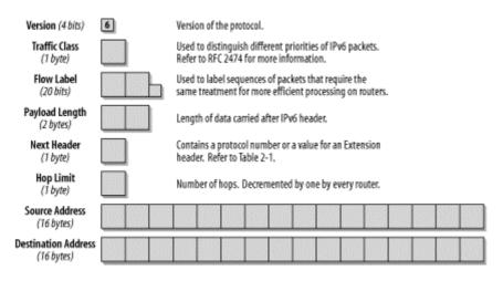
Figure 2-1 shows that even though the header has a total size of 40 bytes, which is twice as long as a default IPv4 header, it has actually been streamlined because most of the header is taken by the two 16-byte IPv6 addresses. That leaves only 8 bytes for other header information.
