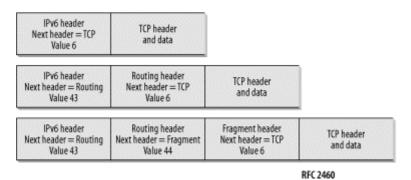
Each Extension header is a multiple of 8 octets long. That way, subsequent headers can always be aligned. If a node is required to process the Next Header but cannot identify the value in the Next Header field, it is required to discard the packet and send an ICMPv6 Parameter Problem message back to the source of the packet. For details on ICMPv6 messages, refer to <u>Chapter 4</u>.
