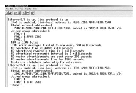
The output shows that I have a link-local address with the prefix FE80 and a global unicast address with the prefix 2002. The multicast group addresses joined are FF02::1 (all nodes), FF02::2 (all routers), and FF02::1:FF0B:75A0 (solicited-node multicast address). A list with all the configuration options follows, stating timers, intervals and address configuration options. Other tools that can be used on Cisco's current IOS are *ping*, *traceroute*, and a DNS client, all operational in IPv6.
