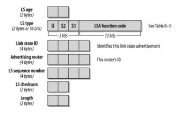
The LSA header fields are fully detailed in the following list:
