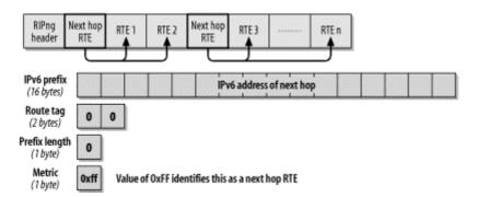
The next hop RTE is identified by a value of  $0 \times FF$  in the metric field of the RTE. The IPv6 address within the RTE is now identified as the next hop IPv6 address to be used by the subsequent RTE. The route tag and the prefix length are set to zero on sending and ignored on reception.
