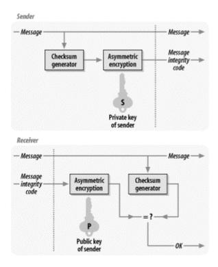
Any recipient of the information and the integrity code can retrieve the sender's public key, use it to decrypt the sender's integrity code, and compare the result to his own checksum calculation. If the results match, the recipient can be sure that the information comes from the intended sender and has not been modified in transit.
