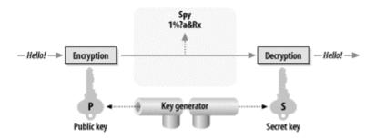
The same mechanism can be used for authentication of information. A sender can calculate a cryptographically secure checksum or hash value for the information to be transmitted, thus creating an integrity code, or electronic signature. The sender then encrypts the resulting integrity code with a private key and transmits it together with the original information (see Figure 5-4).
