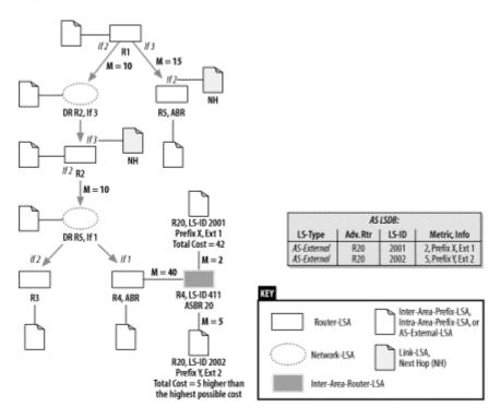
The calculation of the OSPF routing table is now finished, and its content is handed to the internal routing process of the router.
