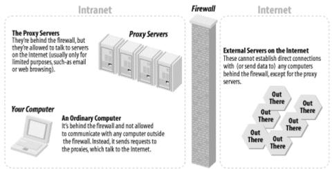
Figure 22-1. The basic firewall architecture
