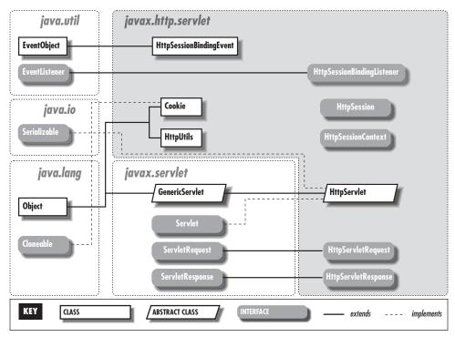
Figure B-1. The javax.servlet.http package
