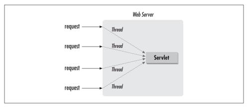
Figure 3-1. Many threads, one servlet instance
