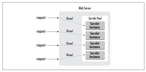
Figure 3-4. The Single Thread Model
