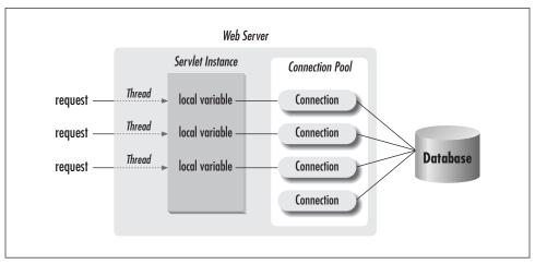
Figure 9-3. Servlets using a database connection pool
