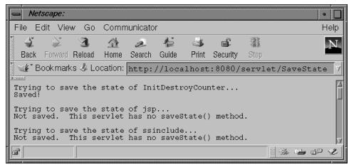
Figure 11-2. Output from the SaveState servlet
