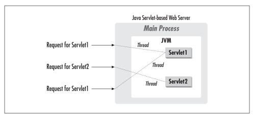
Figure 1-4. The servlet life cycle
