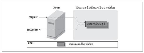
Figure 2-1. A generic servlet handling a request
