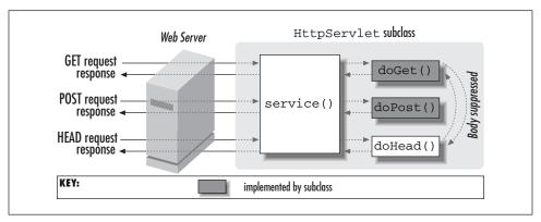
Figure 2-6. An HTTP servlet handling a HEAD request
