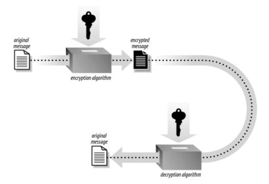
Figure 1-1. Symmetric key cryptography
