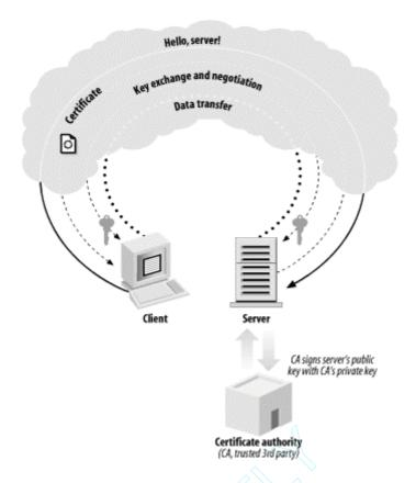
During the connection process, the server will prove its identity by using its private key to successfully decrypt a challenge that the client encrypts with the server's public key. The client needs to receive the correct unencrypted data to proceed. Therefore, the server's certificate can remain public—an attacker would need a copy of the certificate as well as the associated private key in order to masquerade as a known server.
