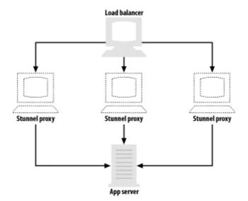
Figure 1-6. Load balancing with Stunnel for cryptographic acceleration
