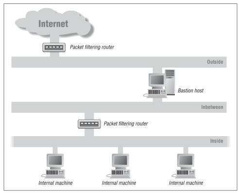
Figure 13-1. Bastion bost configuration
