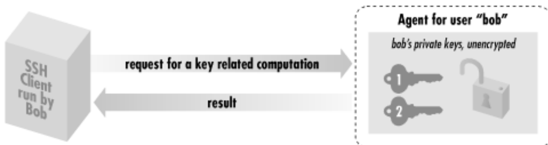
Figure 6.4. How an SSH agent works with its clients
