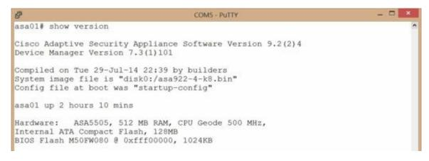
Figure 38: The top of the output of the show version command.
