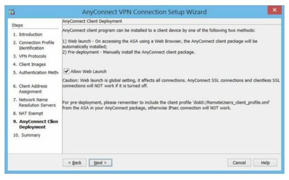
Figure 157: Configuring AnyConnect client deployment
