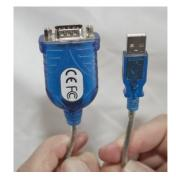
Figure 6: A USB-to-Serial adapter dongle,
