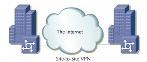
Figure 114: A site-to-site (or lan-to-lan) VPN in which the boxes with arrows represent firewalls connecting two office buildings to the Internet
