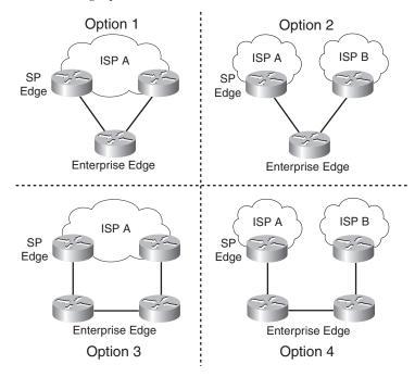
Option 1 provides link redundancy but does not provide ISP and local router redundancy. Option 2 provides link and ISP redundancy but does not provide redundancy for a local router failure. Option 3 provides link and local router redundancy but does not provide for an ISP failure. Option 4 provides for full redundancy of the local router, links, and ISPs.
