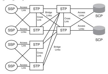
As shown in Figure 15-5, SS7 has the following system components:
