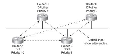
In Figure 11-4, Router A is configured with a priority of 10, and Router B is configured with a priority of 5. Assuming that these routers are turned on simultaneously, Router A becomes the DR for the Ethernet network. Router C has a lower priority, becoming adjacent to Router A and Router B but not to Router D. Router D has a priority of 0 and thus is not a candidate to become a DR or BDR.
