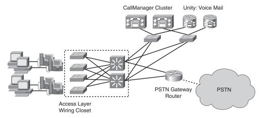
A single CM cluster is deployed for redundancy in the server farm, and Unity is used for voice mail, with or without unified messaging. IP phones are deployed on PoE LAN switches. The Cisco Unified CM supports up to 30,000 IP devices in a cluster. Gateway routers are procured with PRI cards to connect to the enterprise PBX (during migration) or the PSTN.
