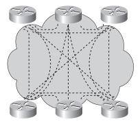
A full-mesh network can be expensive to implement in WANs due to the required number of links. In addition, groups of routers that broadcast routing updates or service advertisements have practical limits to scaling. As the number of routing peers increases, the amount of bandwidth and CPU resources devoted to processing broadcasts increases.
