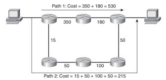
Because the cost of Path 2 is less than that of Path 1, Path 2 is selected as the best route to the destination.
