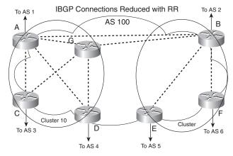
Routers A and G are configured to peer with each other and with Routers B, C, and D. The configuration of Routers C and D is different from the rest; they are configured to peer with Routers A and G only. All route reflectors in the same cluster must have the same cluster ID number.
