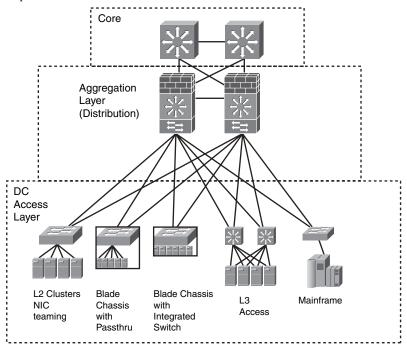
The DC aggregation layer (distribution layer) aggregates traffic to the core. Deployed on the aggregation layer are
