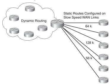
Routing protocols dynamically determine the best route to a destination. When the network topology changes, the routing protocol adjusts the routes without administrative intervention. Routing protocols use a metric to determine the best path toward a destination network. Some use a single measured value such as hop count. Others compute a metric value using one or more parameters. Routing metrics are discussed later in this chapter. The following is a list of dynamic routing protocols:
