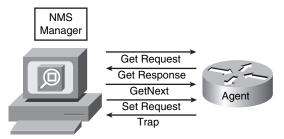
The NMS manager uses the Get operation to retrieve the value-specific MIB variable from an agent. The GetNext operation is used to retrieve the next object instance in a table or list within an agent. The Get Response contains the value of the requested variable.
