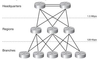
**Figure 2-16** *Partial-Mesh Design with Redundancy*
