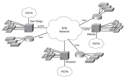
Figure 15-8 Separate Voice and Data Networks
