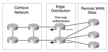
Other locations for one-way redistribution are from building access networks, BGP routes or static routes into the IGP, and from VPN static routes into the IGP.
