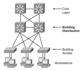
The distribution layer should not be limited on performance. Links to the core must be able to support the bandwidth used by the aggregate access layer switches. Redundant links from the access switches to the distribution layer and from the distribution layer to the core layer allow for high availability in the event of a link failure. Infrastructure services include QoS configuration, security, and policy enforcement. Access lists are configured in the distribution layer.
