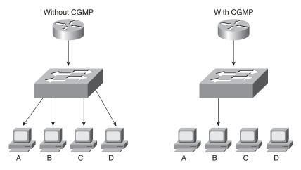
When a router receives an IGMP report, it processes the report and then sends a CGMP message to the switch. The switch can then forward the multicast messages to the port with the host receiving multicast traffic. CGMP fast-leave processing allows the switch to detect IGMP Version 2 leave messages sent by hosts on any of the switch ports. When a host sends the IGMPv2 leave message, the switch can then disable multicasting for the port.
