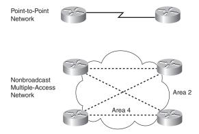
For point-to-point networks, valid neighbors always become adjacent and communicate using multicast address 224.0.0.5. For broadcast (Ethernet) and NBMA networks (Frame Relay), all routers become adjacent to the DR and BDR but not to each other. All routers reply to the DR and BDR using the multicast address 224.0.0.6. The later section "OSPF DRs" covers the DR concept.
