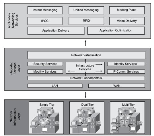
The framework's foundation is the branch profile network infrastructure layer, which includes all the common LAN and WAN components. The integrated services layer is built on top of the infrastructure layer and is composed of security, mobility, UC, and identity services. The application networking services are built above the integrated services layer, which organizes the applications services, such as IM, UCC, unified messaging, video delivery, and application delivery services.
