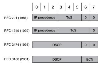
The first 3 (leftmost) bits are the IP precedence bits. These bits define values that are used by QoS methods. The precedence bits especially help in marking packets to give them differentiated treatment with different priorities. For example, Voice over IP (VoIP) packets can get preferential treatment over regular data packets. RFC 791 describes the precedence bits as shown in Table 7-4.
