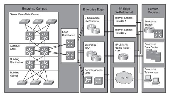
Figure 2-4 Cisco Enterprise Architecture Model
