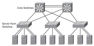
The server-farm switches connect via redundant uplink ports to the core switches. The largest deployments might find it useful to hierarchically construct service to the data center using access and distribution network devices.
