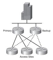
Often, backup links use a different technology. For example, a leased line can be in parallel with a backup dialup line or ISDN circuit. By using *floating static routes*, you can specify that the backup route have a higher administrative distance (used by Cisco routers to select routing information) so that it is not normally used unless the primary route goes down. This design is less available than the partial mesh presented previously. Typically, on-demand backup links reduce WAN charges.
