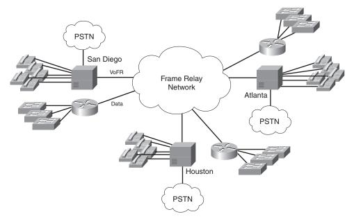
One standard for VoFR is Frame Relay Forum (FRF) 11.1. It establishes specifications for call setup, coding types, and packet formats for VoFR service. It provides the basis for interoperability between vendors.
