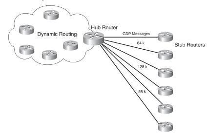
ODR simplifies the configuration of IP with stub networks in which the hub routers dynamically maintain routes to the stub networks. With ODR, the stub router advertises the IP prefixes of its connected networks to the hub router. It does so without requiring the configuration of an IP routing protocol at the stub routers.
