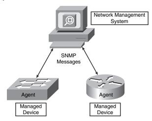
A managed device is a router or LAN switch or any other device that contains an SNMP agent. These devices collect and store management information and make this information available to the NMS. SNMP community strings (passwords) are configured on routers and switches to allow for SNMP management.
