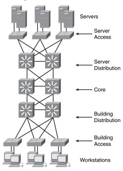
Figure 2-3 Routed Hierarchical Design
