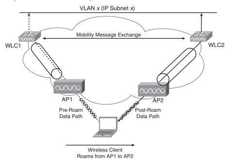
Figure 4-8 Layer 3 Intercontroller Roaming
