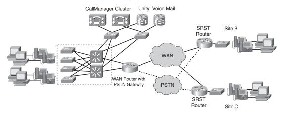
On the WAN, QoS features are configured to prioritize the VoIP packets over other packet types. In the event of WAN failure, SRST configured routers forward calls through the PSTN. The PSTN circuit can be used for local inbound and outbound calls at the remote site. In this model, call admission control (CAC) is configured to impose a limit on the number of on-net calls permitted between sites.
