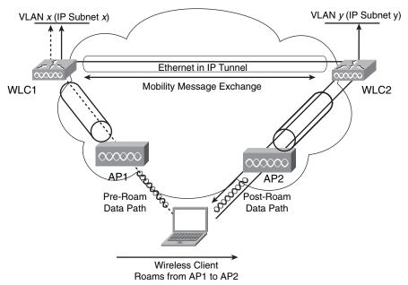
Client traffic then routes in an asymmetric manner. Traffic from the client is forwarded by the Foreign WLC, but traffic to the client arrives at the Anchor WLC, which forwards it through an Ethernet-in-IP (EtherIP) tunnel to the Foreign WLC. The Foreign WLC forwards the data traffic to the client.
