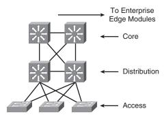
Each layer provides necessary functionality to the enterprise campus network. You do not need to implement the layers as distinct physical entities. You can implement each layer in one or more devices or as cooperating interface components sharing a common chassis. Smaller networks can "collapse" multiple layers to a single device with only an implied hierarchy. Maintaining an explicit awareness of hierarchy is useful as the network grows.
