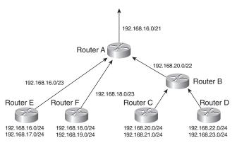
Notice in Table 7-22 that all the Class C networks share a bit boundary with 21 common bits. The networks are different on the 22nd bit and thus cannot be summarized beyond the 21st bit. All these networks are summarized with 192.168.16.0/21.
