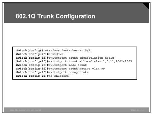
The example shows how to configure interface Fast Ethernet 5/8 as an 802.1Q trunk. Frames from VLANs 1, 5, 11, and 1002 to 1005 will be allowed to traverse the trunk link. The switchport mode for the interface is trunk (on), and no DTP messages will be sent on the interface.
