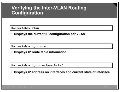
Use the **show** commands to display the current (running) configuration, IP routing information, and IP protocol information. This will verify if the routing table represents the subnets of all VLANs.
