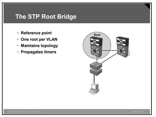
STP uses the concepts of root bridge, root ports, and designated ports to establish a loop-free path through the network. The first step in creating the loop-free spanning tree is to elect a root bridge. The root bridge is the reference point that all switches use to establish forwarding paths that will avoid loops in the Layer 2 network.
