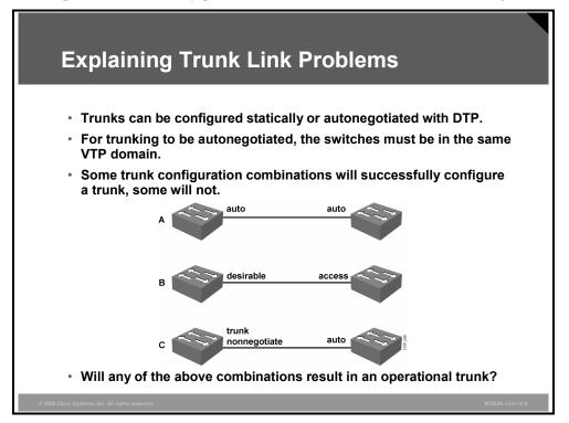
These elements determine whether or not an operational trunk link is formed and also determine the type of trunk the link becomes: the trunking mode, the trunk encapsulation type, the VLAN Trunk Protocol (VTP) domain, and the hardware capabilities of two connected ports.
