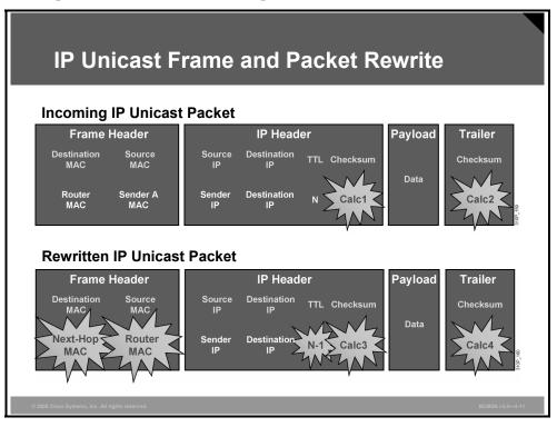
The figure shows how the frame and packet header would be altered when Cisco Express Forwarding (CEF) is used to forward frames. IP unicast packets are rewritten on the output interface as follows:
