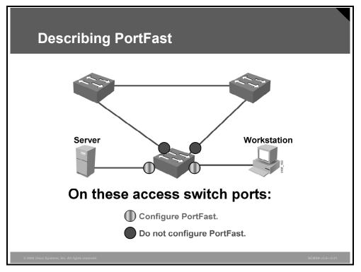
Spanning tree PortFast causes an interface configured as a Layer 2 access port to transition from blocking to forwarding state immediately, bypassing the listening and learning states. You can use PortFast on Layer 2 access ports that are connected to a single workstation or to a server to allow those devices to connect to the network immediately rather than waiting for spanning tree to converge.
