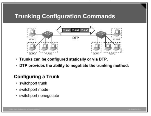
Commands for configuring a trunk will vary, depending on the operating system version of your switch. The commands shown here are for a Cisco IOS software-based switch.
