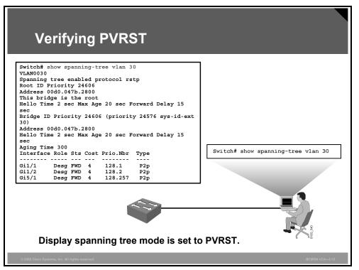
A variety of **show** commands can be used to display configuration and operation information about spanning tree. The **show spanning-tree** command takes several arguments to display a variety of information about the STP configuration. Without any arguments, it will display general information about all STP configurations. The complete syntax is as follows:
