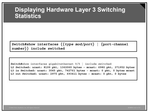
Use the **show interfaces** command with the | *include switch* argument to show switching statistics at each layer for the interface. Verify that Layer 3 packets are being switched.
