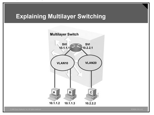
Traditionally, a switch makes forwarding decisions by looking at the Layer 2 header, whereas a router makes forwarding decisions by looking at the Layer 3 header.
