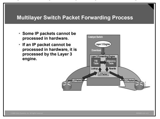
CEF separates the control plane hardware from the data plane hardware and switching. ASICs in switches are used to separate the control plane and data plane, thereby achieving higher data throughput. The control plane is responsible for building the FIB table and adjacency tables in software. The data plane is responsible for forwarding IP unicast traffic using hardware.
