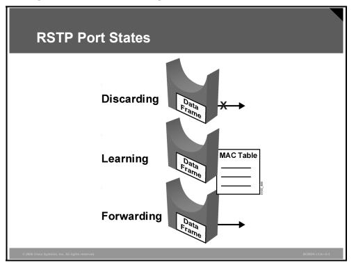
RSTP provides rapid convergence following the failure or re-establishment of a switch, switch port, or link. An RSTP TC will cause a transition in the appropriate switch ports to the forwarding state through either explicit handshakes or a proposal and agreement process and synchronization.
