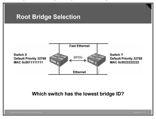
BPDUs are exchanged between switches, and the analysis of the BID and root ID information from those BPDUs determines which bridge is selected as the root bridge.
