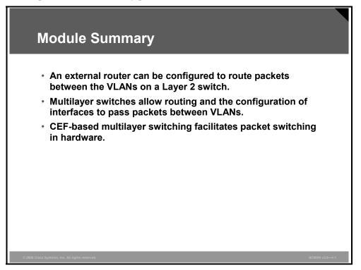
The configuration of multiple Layer 2 VLANs requires that Layer 3 routing occur between those VLANs. This inter-VLAN routing can be provided external to a Layer 2 switch or within a multilayer switch through the configuration of switch virtual interfaces (SVIs) and IP routing.
