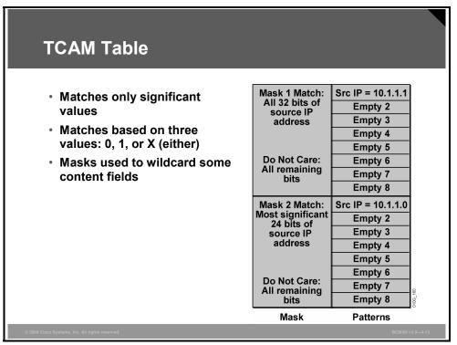
In specific high-end switch platforms, the TCAM is a portion of memory designed for rapid, hardware-based table lookups of Layer 3 and Layer 4 information. In the TCAM, a single lookup provides all Layer 2 and Layer 3 forwarding information for frames, including CAM and ACL information.
