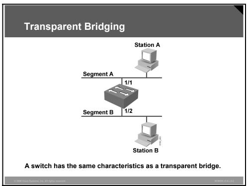
Because switches have replaced bridges as the network device for implementing transparent bridging in modern networks, the basic functionality of a switch is identical to that of a transparent bridge on a per-VLAN basis. To understand STP, it is important first to look at the behavior of a transparent bridge without spanning tree.
