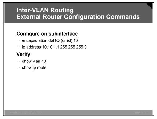
Inter-VLAN routing can be configured using an external router over either ISL or 802.1Q trunks. The commands for configuring the trunk interface on the router are shown in the table.
