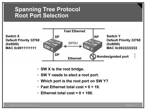
Switch Y receives a BPDU from the root bridge (switch X) on its switch port on the Fast Ethernet segment and another BPDU on its switch port on the Ethernet segment. The root path cost in both cases is zero.
