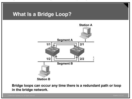
A bridge loop is observed when a frame that is forwarded circulates cyclically and redundantly; this occurs where there is no mechanism to manage the redundant Layer 2 paths.
