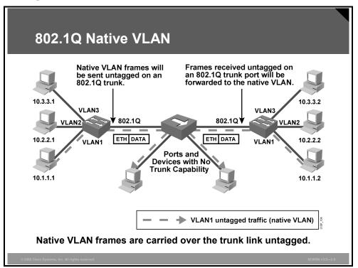
When configuring an 802.1Q trunk, a matching native VLAN must be defined on each end of the trunk link. A trunk link is inherently associated with tagging each frame with a VID. The purpose of the native VLAN is to allow frames that are not tagged with a VID to traverse the trunk link. An 802.1Q native VLAN is defined as one of these:
