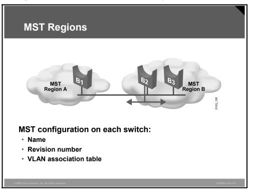
MSTP differs from the other spanning tree implementations in that it combines some, but not necessarily all, VLANs into logical spanning tree instances. This raises the problem of determining what VLAN is to be associated with what instance. More precisely, this means tagging BPDUs so that receiving devices can identify the instances and the VLANs to which they apply.
