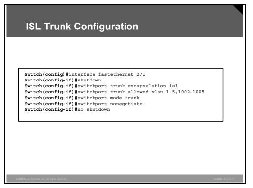
In the example, interface Fast Ethernet 2/1 has been configured as a trunk link for ISL that is permanently on. DTP negotiation is not allowed. The trunk link will carry VLAN traffic for VLANs 1-5 and 1002-1005. VLANs 2-5 are configured on various access ports on the switch, and the trunk links need to carry the frames for these VLANs in addition to the frames for the system VLANs 1002-1005.
