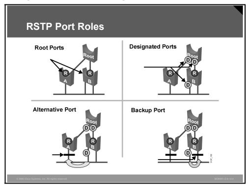
The port role defines the ultimate purpose of a switch port and the way it handles data frames. Port roles and port states are able to transition independently of each other. RSTP uses these definitions for port roles.
