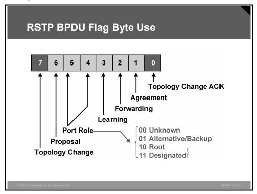
RSTP (802.1w) uses type 2, version 2 BPDUs, so an RSTP bridge can communicate with 802.1D on any shared link or with any switch running 802.1D. RSTP sends BPDUs and populates the flag byte in a slightly different manner than the manner used by 802.1D.
