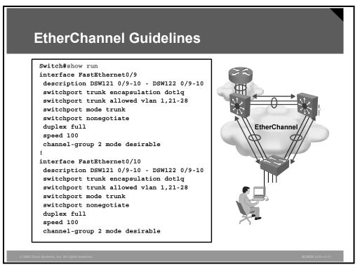
This example shows how to configure an EtherChannel following the guidelines:
