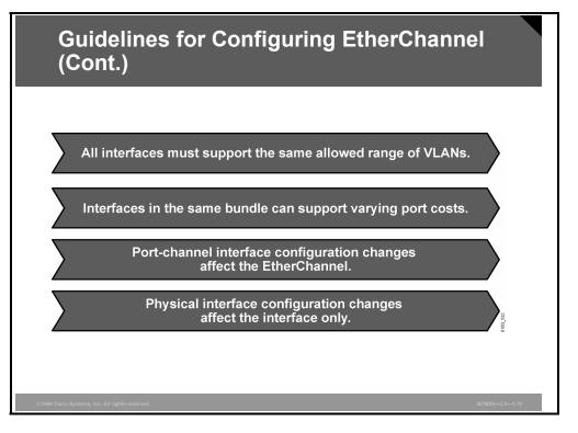
Range of VLANs: An EtherChannel supports the same allowed range of VLANs on all the interfaces in a trunking Layer 2 EtherChannel.
