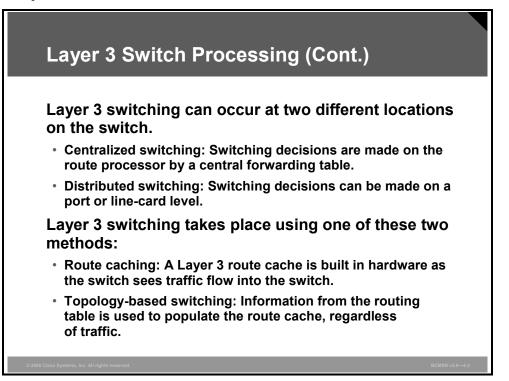
Layer 3 switching can occur at two different locations on the switch.
