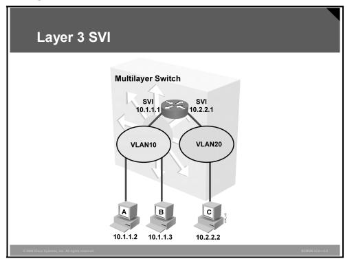
An SVI is a virtual Layer 3 interface that can be configured for any VLAN that exists on a Layer 3 switch. It is "virtual" in that there is no physical interface for the VLAN, and yet it can accept configuration parameters applied to any Layer 3 router interface. The SVI for the VLAN provides Layer 3 processing for packets from all switch ports associated with that VLAN. Only one SVI can be associated with a VLAN. You configure an SVI for a VLAN for these reasons:
