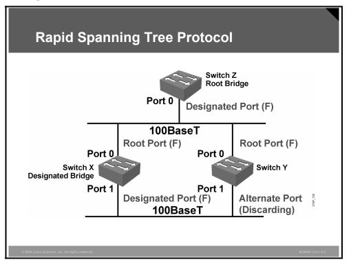
The immediate hindrance of STP is convergence. Depending on the type of failure, it takes anywhere from 30 to 50 seconds to converge the network. RSTP helps with convergence issues that plague legacy STP. RSTP has additional features similar to UplinkFast and BackboneFast that offer better recovery at Layer 2 compared to STP.
