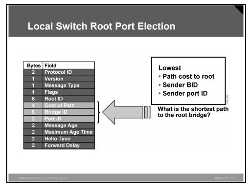
Nonroot bridges place various ports in their proper roles by listening to BPDUs as they come in on all ports. Receiving BPDUs on multiple ports indicates a redundant path to the root bridge.
