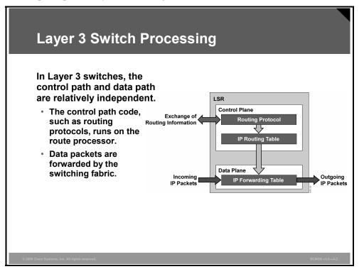
Layer 3 switching refers to a class of high-performance routers optimized for the campus LAN or intranet, providing both wire-speed Ethernet routing and switching services.
