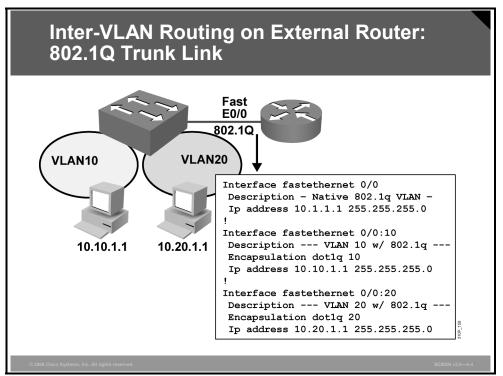
A router interface providing inter-VLAN routing on a trunk link must be configured with a subinterface for each VLAN that will be serviced across the link. Each subinterface on the physical link must then be configured with the same trunk encapsulation protocol. That protocol, either 802.1Q or ISL, is typically determined by what was configured on the switch side of the link.
