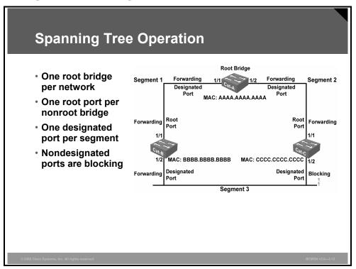
On a nonroot bridge, as spanning tree receives BPDUs on various ports, it determines the roles that each port will fill in the topology. There are four 802.1D port roles.
