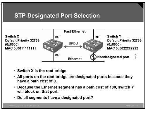
STP selects one designated port per segment to forward traffic. Other switch ports on the segment typically become nondesignated ports and continue blocking, or the switch port could be a root port and continue forwarding, as shown in the figure.
