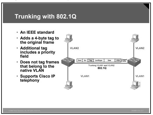
Like ISL, 802.1Q is a protocol that allows a single physical link to carry traffic for multiple VLANs. It is the IEEE standard VLAN trunking protocol. Rather than encapsulating the original Layer 2 frame in its entirety, 802.1Q inserts a tag into the original Ethernet header, then recalculates and updates the FCS in the original frame and transmits the frame over the trunk link.
