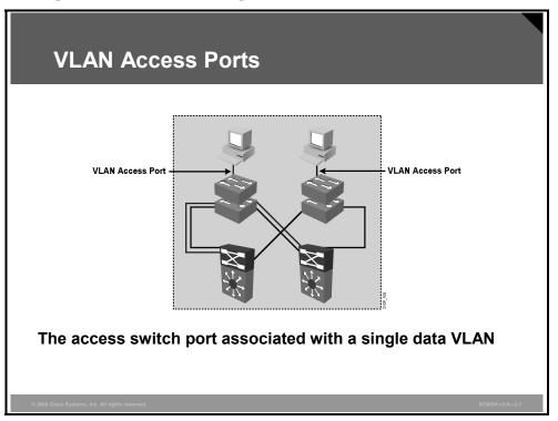
When an end system is connected to a switch port, it needs to be associated with a VLAN, in accordance with the network design. To associate a device with a VLAN, the switch port to which the device connects will be assigned to a single data VLAN and thus becomes an access port. A switch port can become an access port through static or dynamic configuration.
