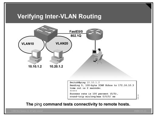
After the router is properly configured and connected to the network, the router or the switch can communicate with other nodes on the network.
