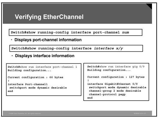
Use the **show interfaces** [*interface*] [*num*] **etherchannel** command to display information about the port channel and the specific EtherChannel interfaces.
