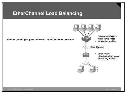
In this figure, an EtherChannel of four workstations communicates with a router. Because the router is a single-MAC-address device, source-based forwarding on the switch EtherChannel ensures that the switch uses all available bandwidth to the router.
