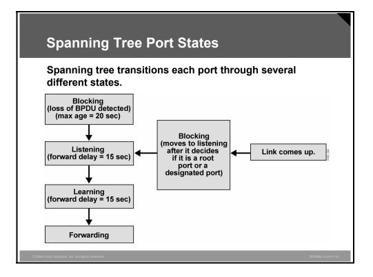
Each Layer 2 port on a switch running STP exists in one of these five port states:
