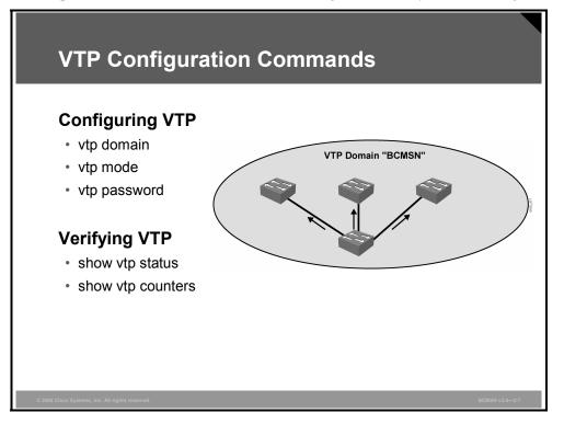
The **vtp** configuration command is used to configure VTP characteristics for a switch. All switches in the same VTP domain will share the same VTP domain name and VTP password, if one is configured. It is a good idea to set the VTP mode to "client" if switches are being added to an existing switched network.
