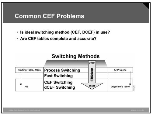
CEF is the fastest means of switching Layer 3 packets in hardware. The CEF tables stored in hardware are populated from information that is gathered by the route processor. Troubleshooting CEF operations therefore has two primary steps.
