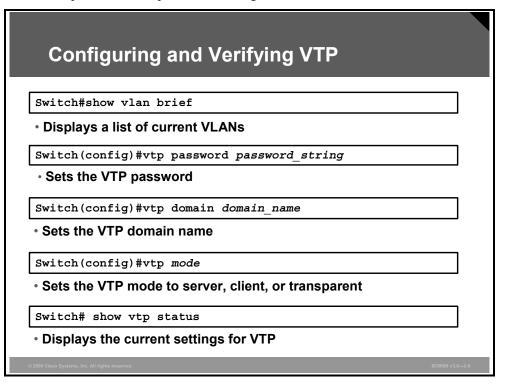
The steps for configuring VTP will vary per design and switch mode, but the general steps for configuring a switch are as follows:
