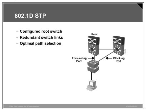
The 802.1D STP provides a mechanism for switches to reconfigure the paths over which they forward frames, making possible a loop-free path when there are redundant switch paths through the network. This is accomplished by forwarding traffic over specific ports and by disabling other ports to prevent frames from being sent repeatedly or in a loop. STP prevents loops by using these mechanisms:
