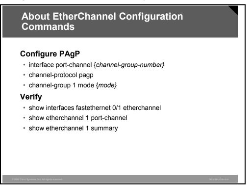
These commands are used to configure and verify EtherChannel.
