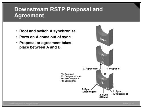
After switch A and the root bridge are synchronized, the proposal and agreement process continues on switch A out of all of its downstream-designated, nonedge ports, as shown in the figure.
