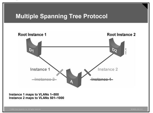
The main purpose of MSTP is to reduce the total number of spanning tree instances to match the physical topology of the network and thus reduce the CPU loading of a switch. The instances of spanning tree are reduced to the number of links (that is, active paths) that are available.
