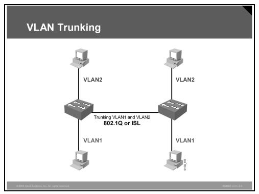
A special protocol is required to establish a trunk link between two devices. A trunk link may exist between these devices:
