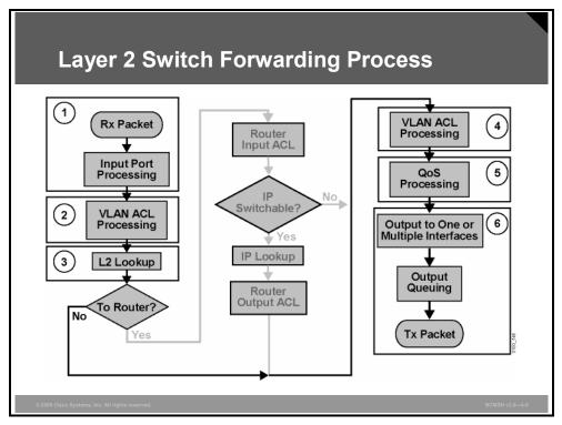
Layer 2 forwarding in hardware is based on the destination MAC address. The Layer 2 switch learns the address, based on the source MAC address. The MAC address table lists MAC and VLAN pairs with associated interfaces.
