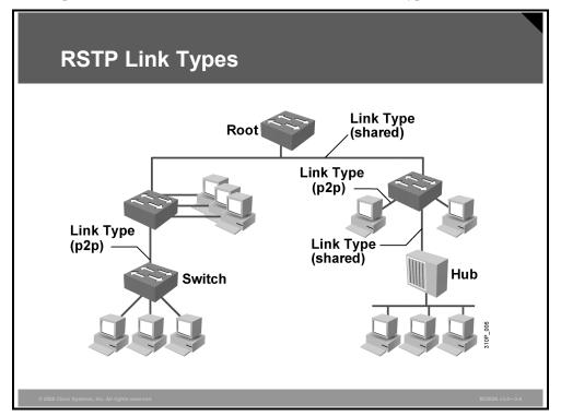
Link type provides a categorization for each port participating in RSTP. The link type can predetermine the active role that the port plays as it stands by for immediate transition to a forwarding state, if certain parameters are met. These parameters are different for edge ports and nonedge ports. Nonedge ports are categorized into two link types. Link type is automatically determined but can be overwritten with an explicit port configuration.
