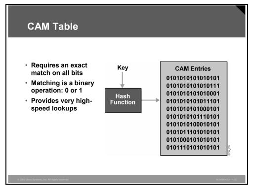
Routing, switching, ACL, and QoS tables are stored in a high-speed table memory so that forwarding decisions and restrictions can be made in high-speed hardware. Cisco Catalyst switches have two primary table architectures:
