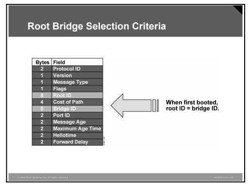
The BID and root ID are both 8-byte fields carried in a BPDU. These values are used to complete the root bridge election process. A switch identifies the root bridge by evaluating the Root ID field in the BPDUs it receives. The unique BID of the root bridge will be carried in the Root ID field of the BPDUs that are sent by each switch in the tree.
