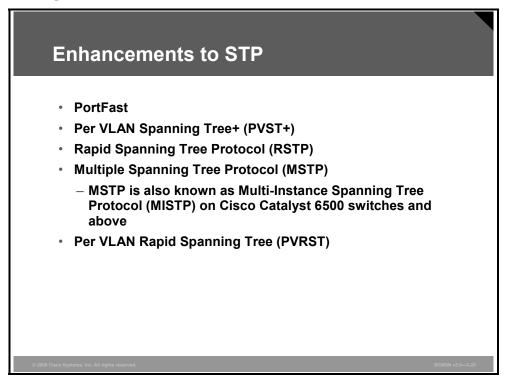
The 802.1D STP standard was developed long before VLANs were introduced. The 802.1D standard has limitations that can be improved by the Cisco Systems proprietary PVST, which allows separate instances of spanning tree and Cisco proprietary features such as PortFast and UplinkFast, which provide much faster convergence.
