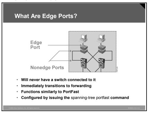
An RSTP edge port is a switch port that is never intended to be connected to another switch device. It immediately transitions to the forwarding state when enabled.
