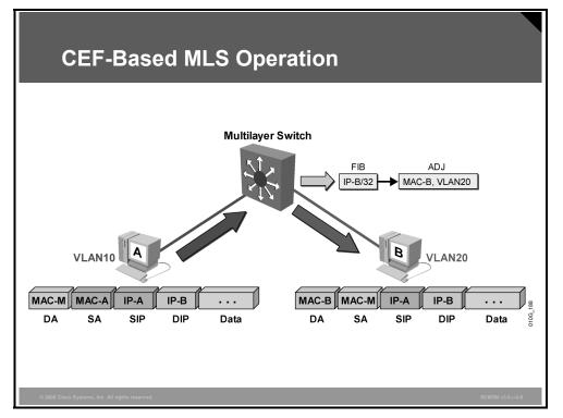
These are the steps that would occur when you use CEF to forward frames between host A and host B on different VLANs.
