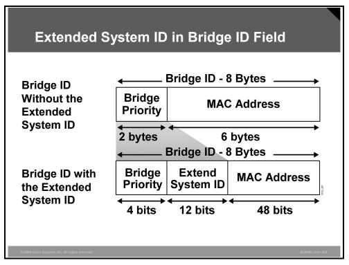
Spanning tree operation requires that each switch have a unique BID. In the original 802.1D standard, the BID was composed of the Priority Field and the MAC address of the switch, and all VLANs were represented by a CST. Because PVST requires that a separate instance of spanning tree run for each VLAN, the BID field is required to carry VLAN ID (VID) information. This is accomplished by reusing a portion of the Priority field as the extended system ID to carry a VID.
