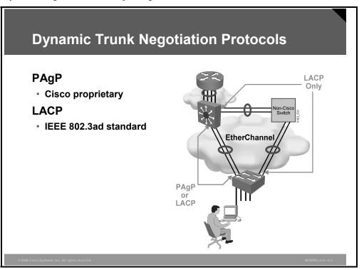
The PAgP aids in the automatic creation of Fast EtherChannel links. PAgP packets are sent between Fast EtherChannel–capable ports to negotiate the forming of a channel. When PAgP identifies matched Ethernet links, it groups the links into an EtherChannel. The EtherChannel is then added to the spanning tree as a single bridge port.
