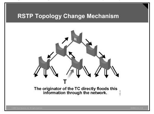
In 802.1D, any port state change generates a TCN. When an 802.1D bridge detects TC, it sends TCNs toward the root bridge. The root bridge sets the TC flag on the outbound BPDUs that are relayed to switches down from the root.
