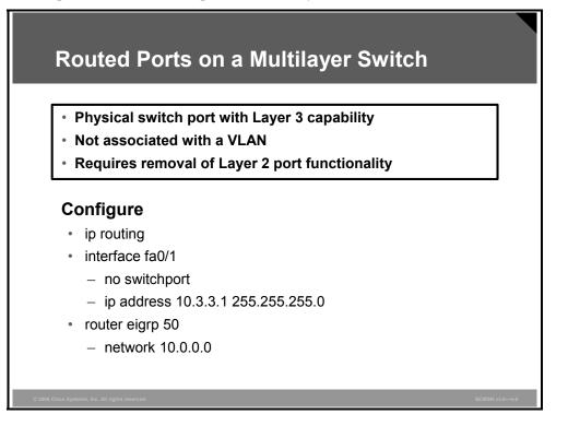
Routed switch ports are typically configured by removing the Layer 2 switch port capability of the switch port. On most switches, the ports are Layer 2 ports by default. On some switches, the ports are Layer 3 ports by default. The layer at which the port functions determines the commands that can be configured on the port.
