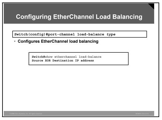
EtherChannel balances traffic load across the links in a channel. The default and the load balancing method varies among the Cisco Catalyst models.
