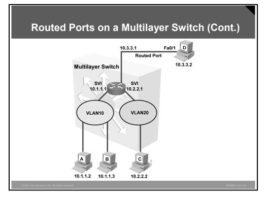
A routed switch port is a physical switch port on a multilayer switch that is capable of Layer 3 packet processing. A routed port is not associated with a particular VLAN, as is an access port or SVI.
