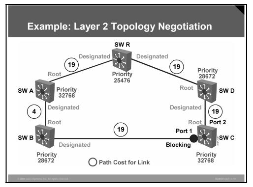
Here is a scenario with switches running STP and exchanging information as shown in the figure. From this information, exchange will yield these final results:
