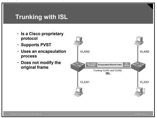
ISL is a Cisco proprietary protocol option for configuring Layer 2 trunk links. It is the original standard for trunking between switches and predates IEEE trunking standards. ISL takes original Layer 2 frames and encapsulates them with a new ISL header and trailer, cyclic redundancy check (CRC), before placing them on the trunk link.
