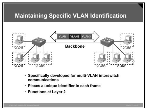
Multiple VLANs are supported between switches through the use of VLAN trunks. A trunk is a Layer 2 link between switches that are running a specialized trunking protocol. Trunks carry the traffic of multiple VLANs over physical links (multiplexing) and enable the extension of a single Layer 2 VLAN between switches.
