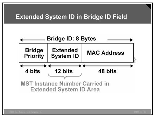
As with PVST, the 12-bit Extended System ID field is used in MSTP. In MSTP, this field carries the MSTP instance number.
