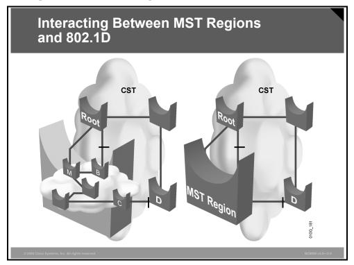
One issue that arises from MSTP design is interoperability with the CST implementation in 802.1D. According to the IEEE 802.1s specification, an MSTP switch must be able to handle at least one Internal Spanning Tree (IST). The MST region consists of one IST and an arbitrary number of MSTP instances.
