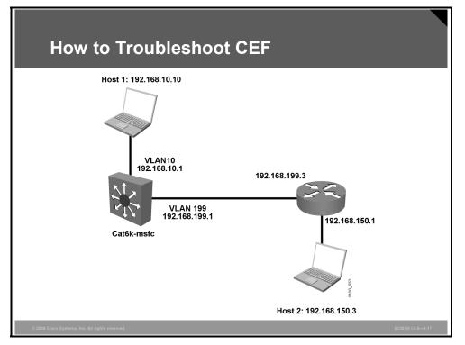
The CEF tables stored in hardware are populated from information that is gathered by the route processor. To properly troubleshoot CEF operations, first ensure that the normal Layer 3 operations on the route processor are functioning properly so that the CEF tables will be populated with accurate and complete information. Next, verify that information from the route processor has properly populated the FIB and adjacency table used by CEF to perform Layer 3 switching of packets.
