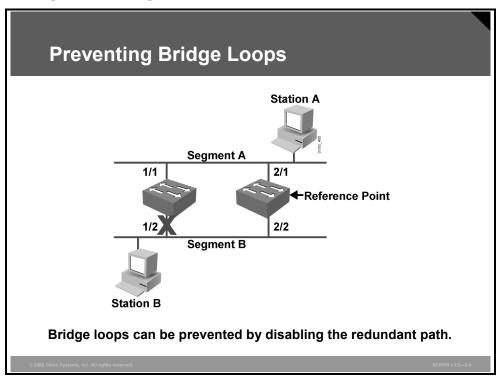
A loop-free network is one in which no Layer 2 loops exist; therefore, the network cannot create Layer 2 broadcast storms or flooded unicast storms. A loop-free network can be achieved manually by shutting down or disconnecting all redundant links between bridges. However, this leaves no redundancy in the network and requires manual intervention in the event of a link failure.
