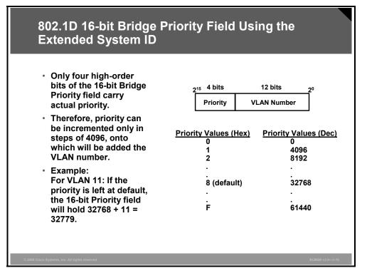
Only four bits are now used to set the bridge priority. Because of the limited bit count, priority is now configurable only in increments of 4096.
