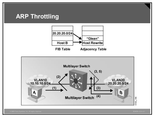
Only the first few packets for a connected destination reach the Layer 3 engine so that the Layer 3 engine can use ARP to locate the host. Throttling adjacency is installed so that subsequent packets to that host are dropped in hardware until an ARP response is received.
