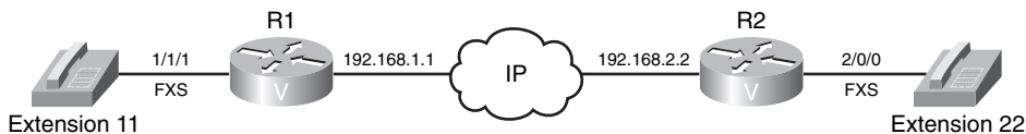
Figure 1-16 Two Sample Voice Gateways with Analog Phones Connected to Their FXS Interfaces
