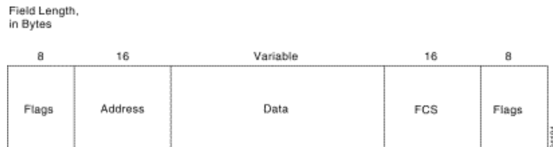
Figure 10-4: Five fields comprise the Frame Relay frame.
