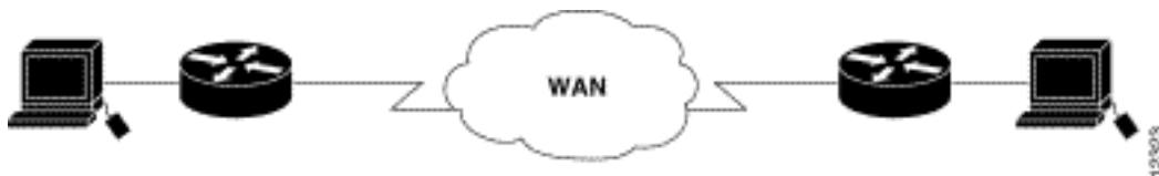
Figure 3-2: A typical point-to-point link operates through a WAN to a remote network.
