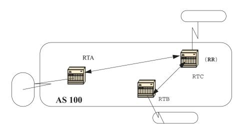
In normal cases, a full IBGP mesh should be maintained between RTA, RTB and RTC within AS100. By utilizing the route reflector concept, RTC could be elected as a RR and have a partial IBGP peering with RTA and RTB. Peering between RTA and RTB is not needed because RTC will be a route reflector for the updates coming from RTA and RTB.
