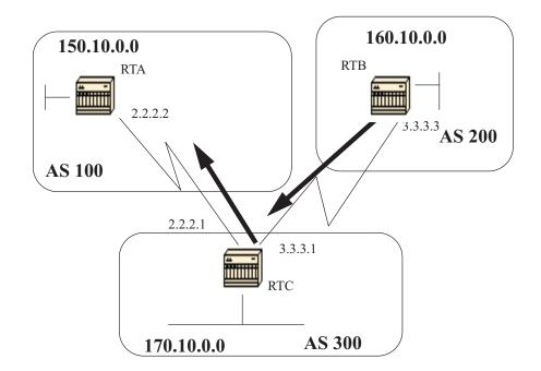
One of the main enhancements of BGP4 over BGP3 is CIDR (Classless Interdomain Routing). CIDR or supernetting is a new way of looking at IP addresses. There is no notion of classes anymore (class A, B or C). For example, network 192.213.0.0 which used to be an illegal class C network is now a legal supernet represented by 192.213.0.0/16 where the 16 is the number of bits in the subnet mask counting from the far left of the IP address. This is similar to 192.213.0.0 255.255.0.0.
