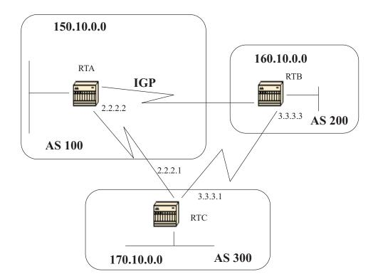
Consider the above diagram, RTA and RTC are running EBGP and RTB and RTC are running EBGP. RTA and RTB are running some kind of IGP (RIP, IGRP, etc.)
