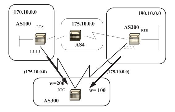
The weight attribute is a Cisco defined attribute. The weight is used for a best path selection process. The weight is assigned locally to the router. It is a value that only makes sense to the specific router and which is not propagated or carried through any of the route updates. A weight can be a number from 0 to 65535. Paths that the router originates have a weight of 32768 by default and other paths have a weight of zero.
