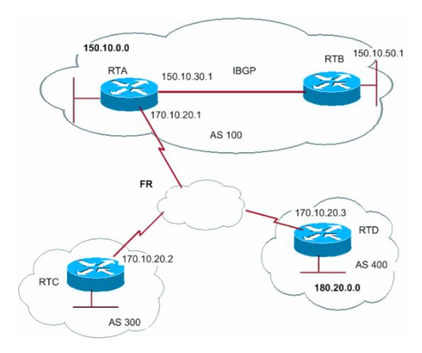
The common medium appears as a cloud in the diagram. If the common medium is a frame relay or any NBMA cloud, the exact behavior is as if you have connection via Ethernet. RTC advertises 180.20.0.0 to RTA with a next hop of 170.10.20.3.
