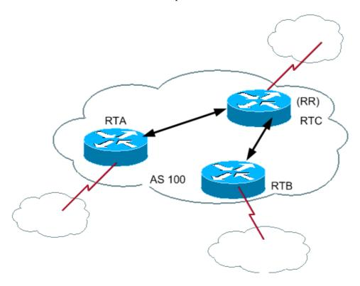
In normal cases, maintain a full iBGP mesh between RTA, RTB, and RTC within AS100. If you utilize the RR concept, RTC can be elected as an RR. In this way, RTC has a partial iBGP peering with RTA and RTB. Peering between RTA and RTB is not necessary because RTC is an RR for the updates that come from RTA and RTB.
