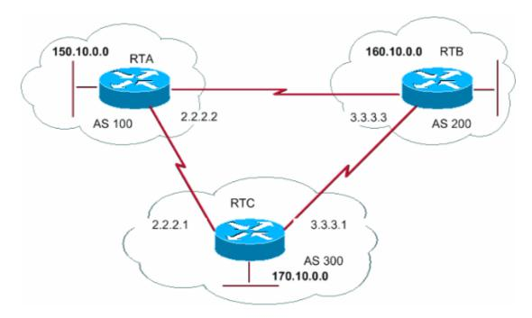
In this diagram, RTA and RTC run eBGP. RTB and RTC run eBGP. RTA and RTB run some kind of IGP, either RIP, IGRP, or another protocol. By definition, eBGP updates have a distance of 20, which is less than the IGP distances. The default distances are:
