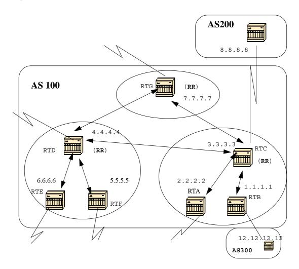
An autonomous system can have more than one route reflector; a RR would treat other RRs just like any other IBGP speaker. Other RRs could belong to the same cluster (client group) or to other clusters. In a simple configuration, the AS could be divided into multiple clusters, each RR will be configured with other RRs as non-client peers in a fully meshed topology. Clients should not peer with IBGP speakers outside their cluster.
