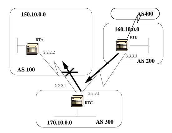
You can specify an access list on both incoming and outgoing updates based on the BGP autonomous system paths information. In the above figure we can block updates about 160.10.0.0 from going to AS100 by defining an access list on RTC that prevents any updates that have originated from AS 200 from being sent to AS100. To do this use the following statements.
