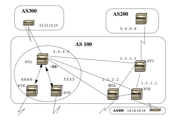
In the above diagram, RTD, RTE and RTF have the concept of route reflection. RTC, RTA and RTB are what we call conventional routers and cannot be configured as RRs. Normal IBGP mesh could be done between these routers and RTD. Later on, when we are ready to upgrade, RTC could be made a RR with clients RTA and RTB. Clients do not have to understand the route reflection scheme; it is only the RRs that would have to be upgraded.
