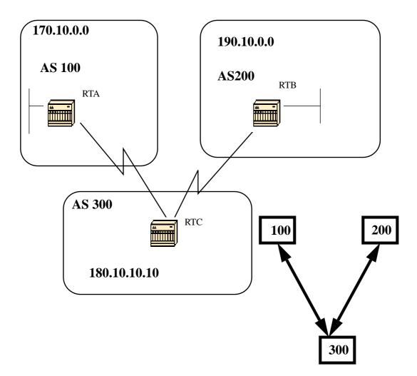
Whenever a route update passes through an AS, the AS number is prepended to that update. The **AS\_path** attribute is actually the list of AS numbers that a route has traversed in order to reach a destination. An **AS-SET** is an ordered mathematical set {} of all the ASs that have been traversed. An example of AS-SET is given later.
