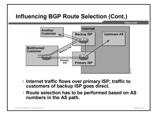
In most cases, it is more optimal to reach other customers connected to the backup ISP via the backup link, compared with reaching them via the primary link.
