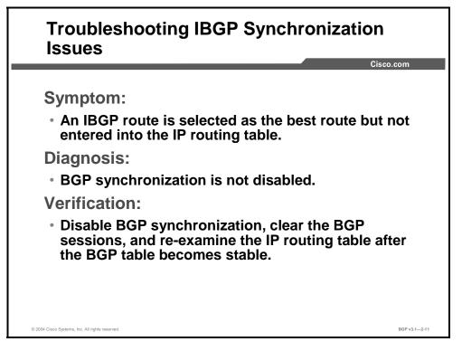
In old BGP designs, redistribution between BGP and an IGP was common practice, and these protocols had to be synchronized to ensure proper packet forwarding. In modern designs, redistribution is no longer used and the synchronization has to be turned off. However, the default value is to have synchronization enabled.
