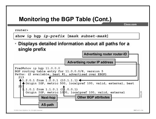
If more information and the complete set of BGP attributes are required, the **show ip bgp** command should be entered with the network number on the command line. This command displays all relevant BGP information about that specific network.
