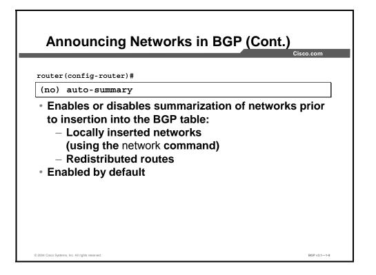
When the router is configured to locally announce routes into BGP, the behavior of the **network** command varies depending on whether automatic summarization is enabled or disabled. When automatic summarization is enabled, the command summarizes locally originated BGP networks to their classful boundaries. By default, automatic summarization is enabled for BGP.
