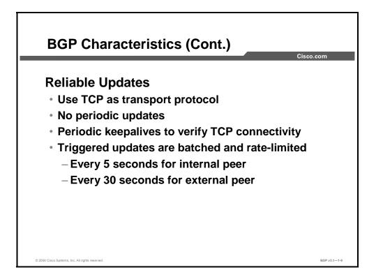
The reliable transport mechanism that is used by BGP is standard TCP. BGP is an application protocol that uses both the TCP and IP protocols for reliable connections.
