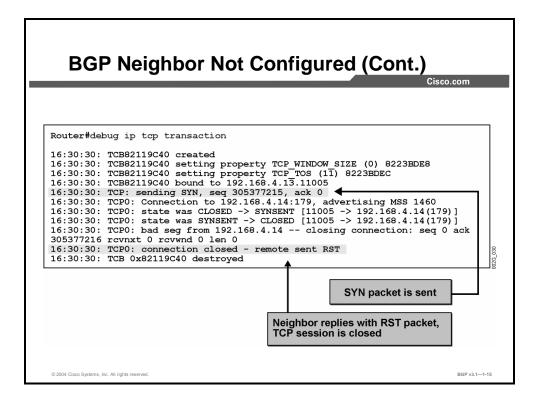
In the example here, the remote router is not configured for BGP or there was a mismatch in the neighbor IP addresses. The remote router responds with an RST packet as soon as it receives the initial SYN packet, terminating the BGP session.
