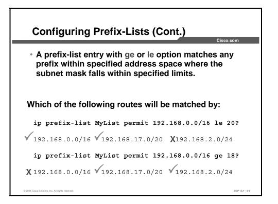
Prefix-list entries with the **ge** or **le** option specified match any prefix within the address space that is specified by the *network/len* parameter, as long as the subnet mask length of the route falls within the range that is specified by the **le** and **ge** parameters.
