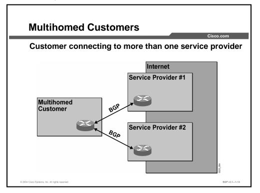
The figure illustrates a customer network that is connected to two different ISPs, which requires the use of BGP for full redundancy.
