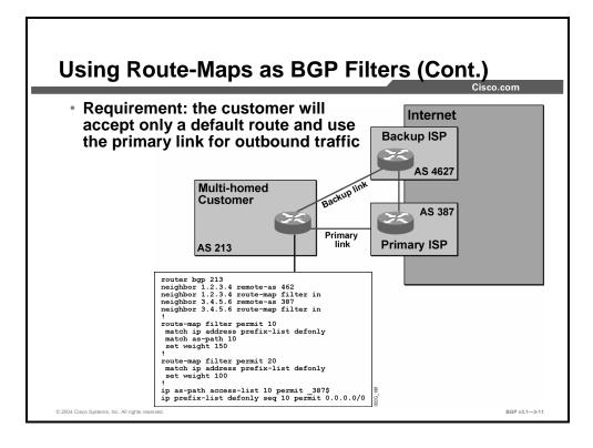
In this example, the customer will accept only a default route and use the primary link that is connected to AS 387 for outbound traffic.
