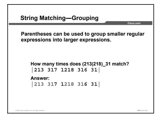
Complicated expressions must sometimes be grouped with parentheses, "(" and ")". This feature can be useful when you are searching for a sequence of two or more AS numbers of which the first can match any of the specific autonomous systems (in this example, "213" or "218"), but the last must be a specific AS ("31" in this example). If the parentheses were not used here, the expression would match either the single AS "213" or the sequence of the two "218 31".
