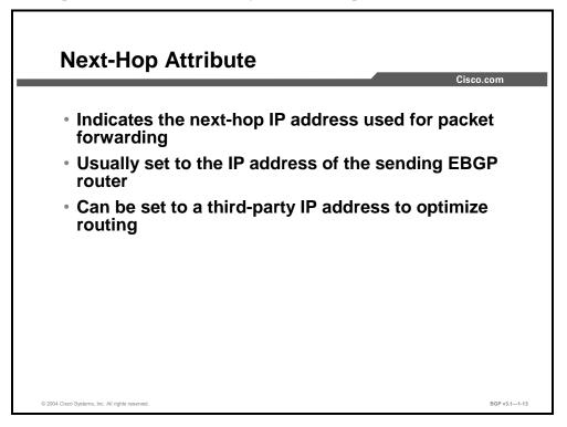
The BGP next-hop attribute identifies the IP address that a router should use to forward packets toward the destination that is announced in a BGP routing update. In most cases, the sending router sets the next-hop attribute to its own IP address. There are cases, however, where the next-hop IP address points to a third router.
