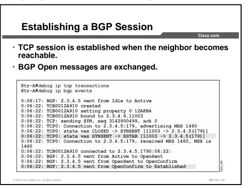
Before any connection attempt is made, the BGP peer relation must have left the Idle state and entered the Active state. For a BGP session between two routers in different autonomous systems, this situation happens when the IP address of the remote router becomes reachable on a directly connected interface.
