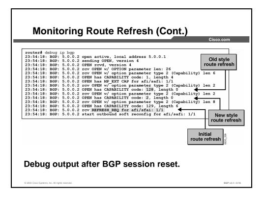
Use **debug ip bgp** to display the negotiation of capabilities. Debugging displays received capabilities.
