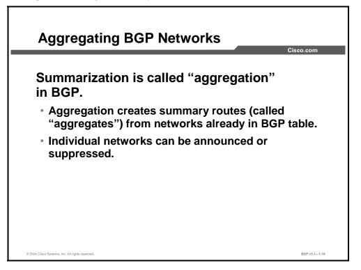
When the BGP table is already populated with routes that should be summarized, you must configure a router to do so. The summarization of BGP routes is called "aggregation."
