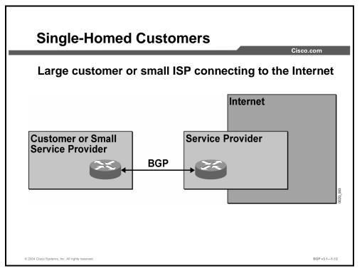
The figure shows a customer network connected to the Internet using a single ISP, but such a scenario is generally not the case when BGP is used. Normal Internet access to a single ISP does not require BGP; static routes are more commonly used to handle this situation. Small ISPs buying Internet connectivity from other ISPs use this type of connectivity more often, especially if they want to start their business the proper way-by using their own AS number and having their own address space.
