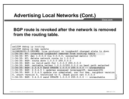
In this example, network 1.0.0.0/8 is directly connected to interface Loopback0. The route to 1.0.0.0/8 has been previously installed in the BGP table because it was listed with a network statement and it was in the routing table as directly connected. When the Loopback0 interface goes down, the router removes the directly connected route from its routing table. Because the route no longer exists in the routing table, it must also be removed from the BGP table.
