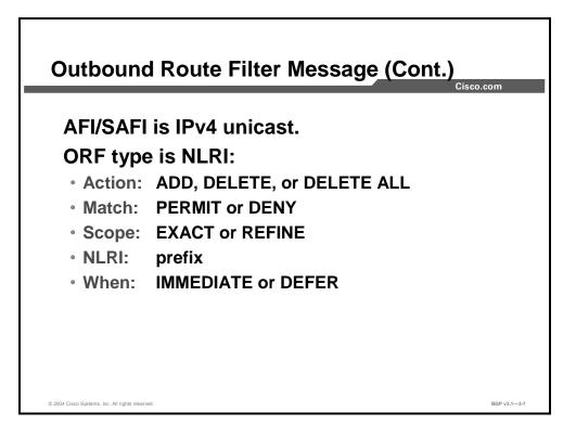
The content of the ORF value is determined by the ORF-type setting. An ORF type of NLRIbased filtering (type 1) uses the following actions:
