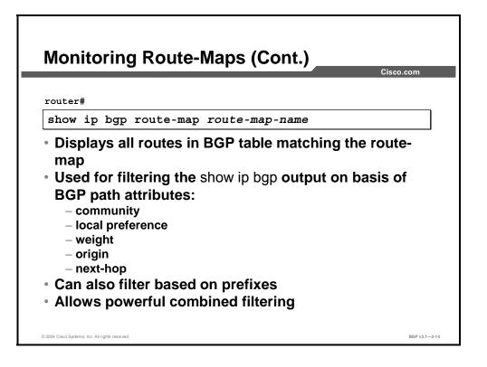
You can also use route-maps for selective and powerful filtering of the BGP table. The **show ip bgp route-map** command displays selected routes from a BGP routing table based on the contents of a route-map.
