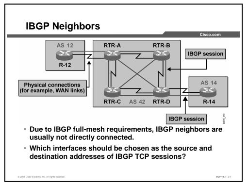
In this example, the transit AS 42 has a redundant physical topology. The IGP provides reachability information for all routers and networks within AS 42, allowing all routers in the AS to establish IBGP sessions to all other routers, even if not directly connected.
