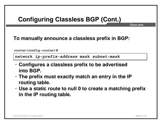
To advertise classless networks into BGP (a subnet or a supernet), you can use the **network** command with the **mask** keyword and the subnet mask specified. When an exact match is not found in the IP routing table (for example, when you are creating a summary or when you are advertising only a part of your address space), a matching prefix has to be manually configured on the router in the form of a static route pointing to the null 0 interface; otherwise, the advertisement will not succeed.
