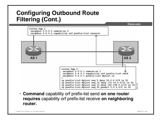
The example shows the configuration of two routers where one router has uploaded an input prefix-list to the neighbor to be used as an output filter.
