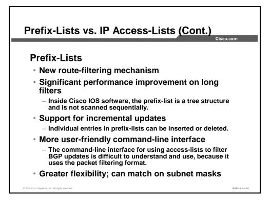
The **ip prefix-list** configuration command has several benefits compared to using the **access-list** command. The intended use of prefix-lists is limited to route filtering, whereas access-lists were initially intended for packet filtering, which was then extended to filter routes.
