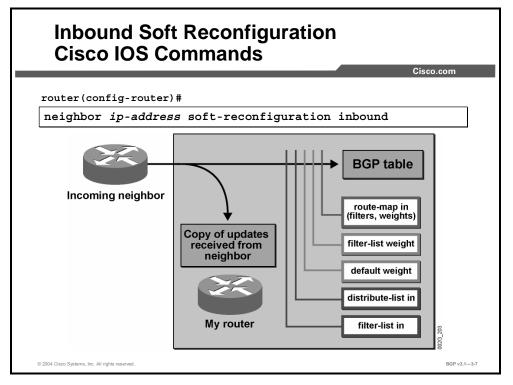
When you configure **soft-reconfiguration inbound** for a neighbor, the router stores all routes that are received from that neighbor as an extra copy in memory. This copy is taken before any filtering is applied by the router to routes that it receives.
