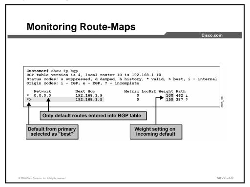
Use the **show ip bgp** command to display the configured route-map characteristics.
