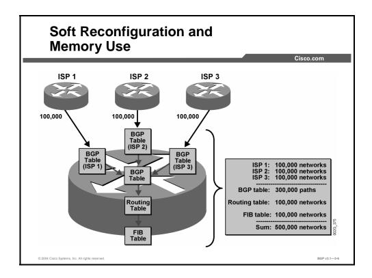
This example shows the impact of soft reconfiguration on an ISP router with three upstream neighbors sending full Internet routing information.
