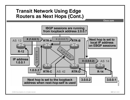
The next-hop attribute is normally not changed on IBGP updates. In the figure, the **next-hop-self** configuration has been used on all IBGP sessions. When the border router forwards the incoming EBGP update over an outgoing IBGP session, the border router changes the next-hop address to the IP address that is used as the source address of the IBGP session.
