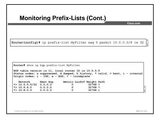
This example shows a simple prefix-list-based filtering of the BGP table. The prefix-list filter permits all networks with the first octet equal to 10 and any length of a subnet mask (**le 32**). In the **show ip bgp prefix-list** output, only the networks permitted by the prefix-list filter are displayed.
