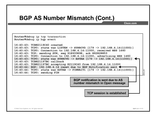
Whenever there is a mismatch in AS numbers (or any other BGP parameters that are necessary for proper BGP operation), the BGP session is terminated with a BGP notification, and the TCP session is terminated as well.
