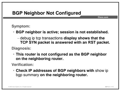
If the TCP SYN packet is answered with a TCP RST packet, the remote router is alive and reachable but is not willing to grant the connection attempt. The reason for this refusal may be that BGP has not been fully configured on the remote router or that the source IP address that is used by the local router in the connection attempt is not in the list of valid neighbors for the remote router.
