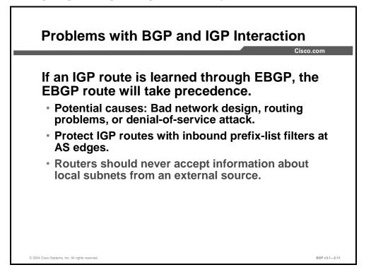
If routing information about the same IP prefix is learned via both EBGP and an IGP, the router will use the EBGP information. If an external AS is feeding the local AS with EBGP routes that actually should be local, routers within the AS will erroneously forward IP packets that are destined to those local networks out of the local AS.
