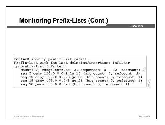
In this example, the **show ip prefix-list** command has been issued with the **detail** keyword. The output of the command displays detailed information about configured prefix-lists, including sequence numbers, the prefix-list entries, and the number of times that each entry has been matched by a corresponding prefix.
