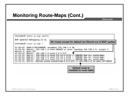
Here we see that all routes except for the default route are being filtered out (DENIED) of the BGP update. The default route is installed in the route table.
