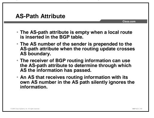
The AS-path attribute is modified by an edge router every time information about a particular IP subnet passes over an AS border. When a router first originates a route in BGP, the AS-path attribute is empty. The local AS number is prepended to the AS path each time that the route crosses an AS boundary. There are several consequences of this behavior:
