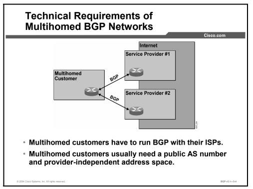
The multihomed customer network must exchange BGP information with both ISP networks. Dynamic routing is required for full redundancy, and BGP is the only protocol available that can be used in this scenario.
