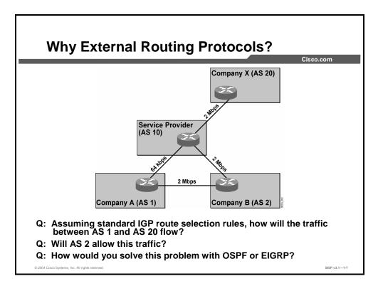
The figure illustrates the need for an interdomain routing protocol. It depicts two companies that are connected to the Internet via leased lines of differing speed.
