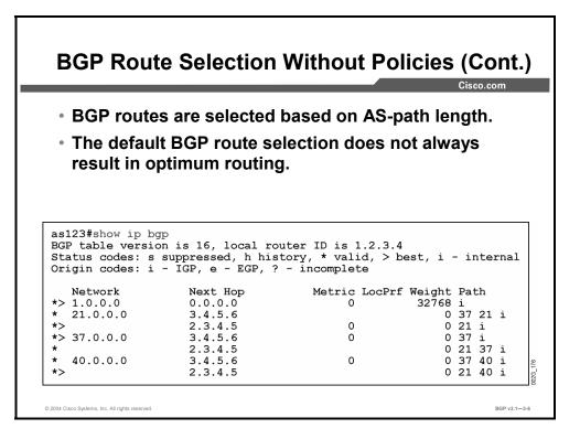
This is an example of a multihomed customer with AS 123. It is connected to two different ISPs: AS 37 and AS 21. The two ISPs are interconnected, and both are also connected to AS 40.
