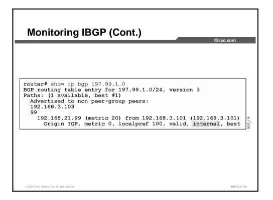
The **show ip bgp** *prefix* command displays whether a BGP route was received from an IBGP (internal) or EBGP (external) neighbor. The indication is given by the word "internal" that is displayed in the last line of the printout (marked white in the last line of the figure).
