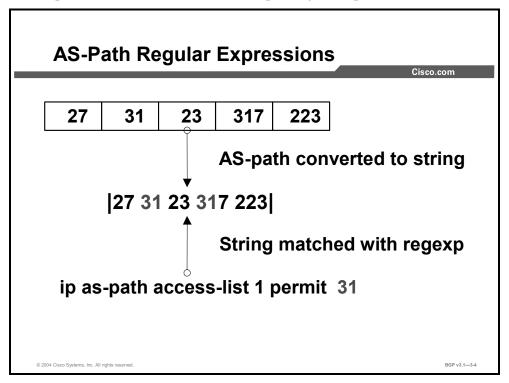
The AS-path attribute carried with all BGP routes in a BGP update is a very compact binary encoding of a sequence of integer numbers. It is not a sequence that can be tested by using a regular expression.
