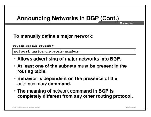
To specify the networks to be advertised by the BGP routing process, use the network router configuration command. To remove an entry, use the **no** form of this command.
