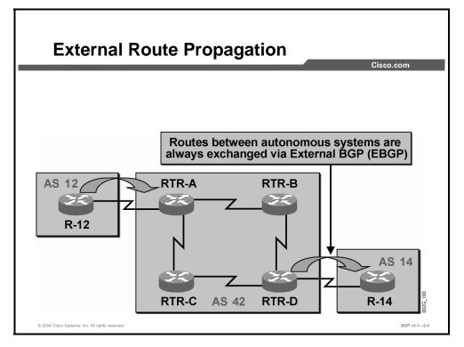
Two autonomous systems usually exchange routing information about reachable networks using BGP. There is currently no alternative routing protocol that has the scalability and security characteristics of BGP.
