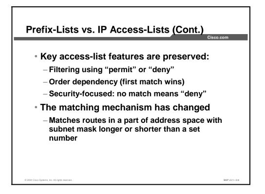
The prefix-list has several similarities with the access-list. It can consist of any number of lines, each of which indicates a test and a result. The router can interpret the lines in the specified order, although this is optimized in the Cisco IOS software. When a router evaluates a route against the prefix-list, the first line that matches will result in either a "permit" or "deny." If none of the lines in the list match, the result is "implicitly deny."
