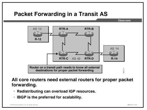
When BGP updates have propagated through the transit AS to all neighboring autonomous systems, the IP traffic can start to flow.
