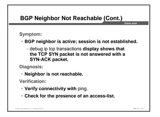
TCP session establishment starts with the router sending a TCP SYN packet. If the TCP SYN packet is never answered, the remote router might be dead or not reachable. Try to use the **ping** command and verify the existence of the remote router and the IP packet exchange between the local and remote router.
