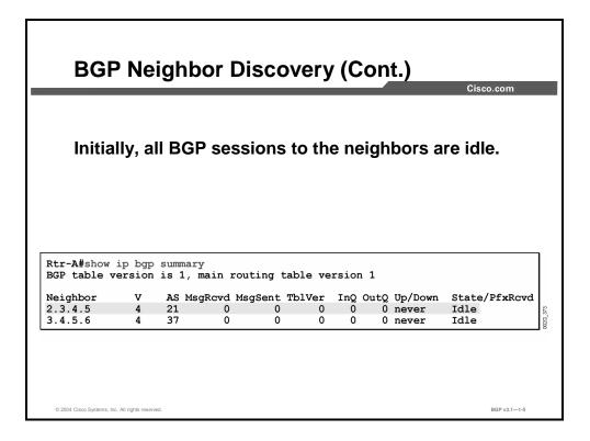
The show ip bgp summary command gives an overview of the BGP status. Each configured neighbor is listed in the output of the command. The IP address to which the connection attempts are directed is also displayed, along with BGP version number, the remote AS number, some counter values, the status of the session, and how long ago the session changed state.
