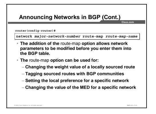
When the router is configured to insert routes in the BGP table, the default attributes of locally sourced routes can be modified with the inclusion of the **route-map** option in the basic **network** command.
