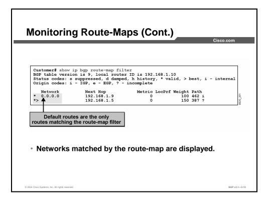
In this example, a customer is using a simple route-map to filter the BGP table. By using the show ip bgp route-map command, the customer can display the filtered BGP table. The customer router configuration from which this output is collected is shown here for reference:
