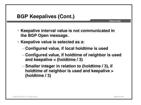
As opposed to the holdtime interval, BGP peers do not communicate the keepalive interval in the Open message. The selection of a keepalive interval is therefore based on the selected holdtime value. The selected holdtime value that is used by both peers is the smaller one of both configured values.
