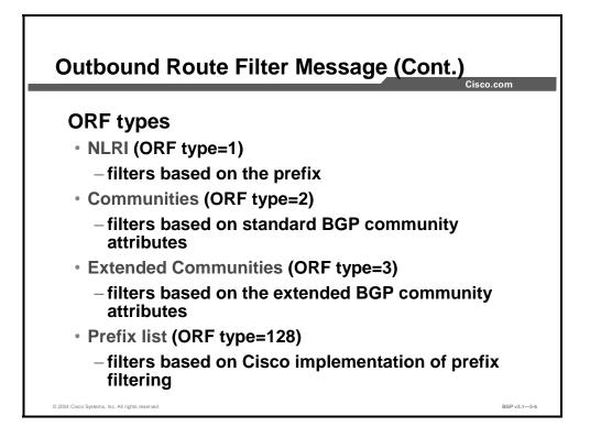
The value contained in the ORF type determines the content that is contained in the ORF message.
