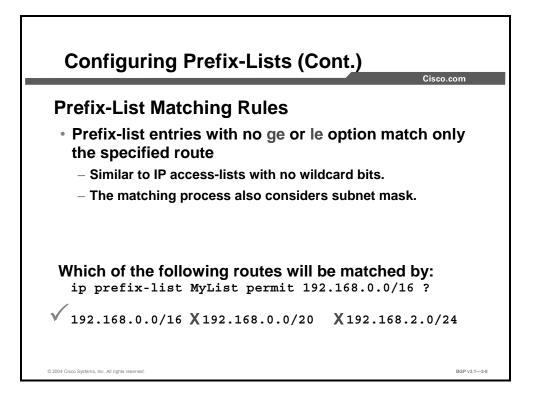
Prefix-list entries without the **ge** or **le** option match only the route with the specified IP address and subnet mask. In the example here, the prefix-list entry **permit 192.168.0.0/16** will not match the route 192.168.2.0/24 because of the mismatch in the IP address. It will also not match the route 192.168.0.0/20 because of the mismatch in the subnet mask.
