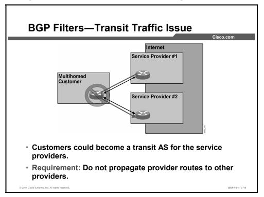
When BGP has selected the best path, the information is advertised by the router to all neighboring autonomous systems, except for the session that it was received on (called "BGP split-horizon functionality," preventing near-range routing loops). This situation causes the customer AS to become a transit AS between the two ISPs, and should be avoided.
