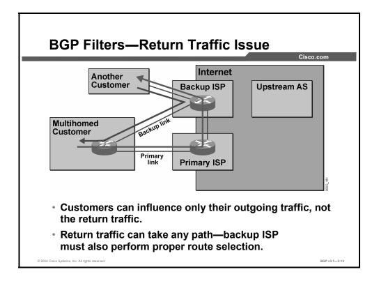
The customer can easily define a policy about how to send outgoing IP packets on the correct link. It is much harder to influence the neighboring AS about how to direct the IP packets coming into the customer network.
