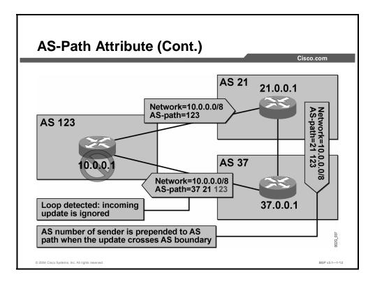
The figure shows how BGP loop prevention works.
