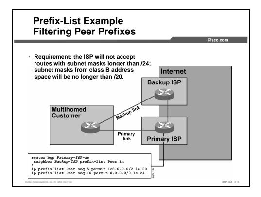
In this example, the primary ISP will not accept any route from the customer that indicates a subnet smaller than a 255.255.255.0 subnet mask. The class B network, however, must not be subnetted into smaller subnets than a 255.255.240.0 subnet mask.
