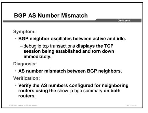
If the TCP session is established using the specified three-way handshake of SYN, SYN-ACK, and ACK, but the router drops the session after a short packet exchange, the BGP parameters are mismatched. Make sure that the remote AS that is configured on the router matches the local AS that is configured on the neighbor. If the AS numbers do not match, the router will drop the session after exchanging BGP Open messages.
