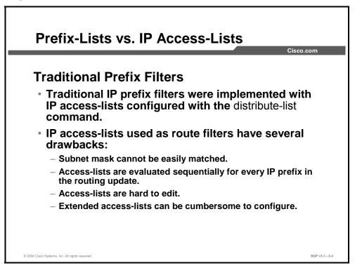
Traditionally, filtering of IP network numbers has been accomplished using an access-list. The access-list is then bound to either the incoming or outgoing information of a neighbor by the **neighbor distribute-list** command. A BGP update about a network number that is permitted by the access-list will be accepted, and those denied will be dropped.
