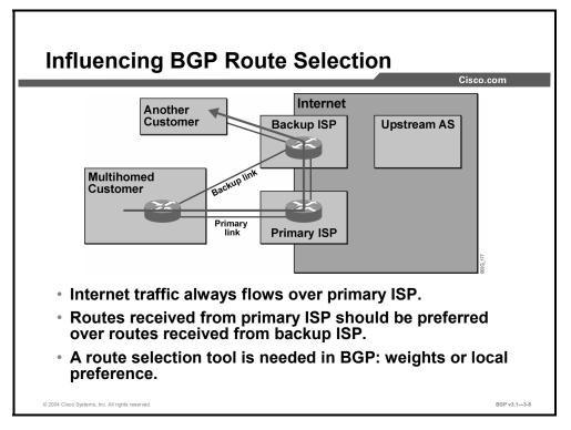
When one of the two ISPs is designated as a primary ISP and the other a backup, BGP attributes must be configured as a means of influencing BGP route selection rules. If both ISP connections terminate in one single customer router, all routes that are received from the primary ISP can be assigned a BGP weight. A higher weight indicates a more preferred path.
