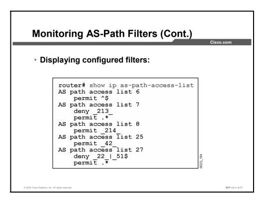
The **show ip as-path-access-list** command displays a specific access-list or all AS-path access-lists in the router.
