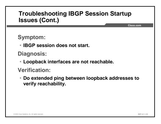
An IBGP session between two routers can be established from the loopback interface of one router to the loopback interface of the other router only if the two routers can exchange IP packets using those addresses as source and destination. This exchange is possible only if the IGP carries the subnets that are assigned to each of the loopback interfaces.
