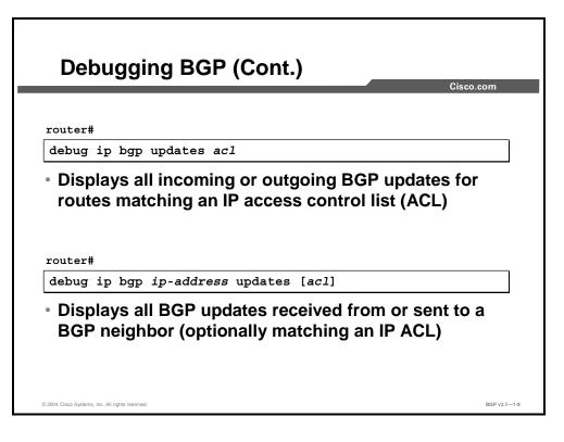
To avoid debug printouts for every update that is sent or received, you can create and associate an access-list with the **debug** command. When you use this command, the console will display only the updates that refer to a network number that is permitted by the access-list. The command is extremely useful in a live network with busy BGP sessions where the troubleshooter is interested only in updates for specific networks.
