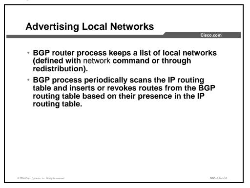
The BGP routing process can inject new routes in the BGP table. A router will propagate newly injected routes to neighboring BGP peers if it selects them as best, giving neighboring autonomous systems information about networks that are reachable in the local AS. This process is called advertising, originating, or announcing, local routes.
