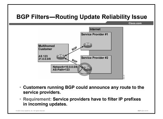
Without some sort of filtering, BGP routing information that is created by the AS of the customer can potentially be propagated all over the Internet. In this way, the customer can inject erroneous information into the Internet routing tables.
