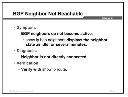
BGP sessions to a router in another AS should normally run across directly connected interfaces (routers that share a common IP subnet). You must configure neighboring routers to reach each other using the IP address belonging to this shared subnet so that no other routing protocol is required to set up the BGP session.
