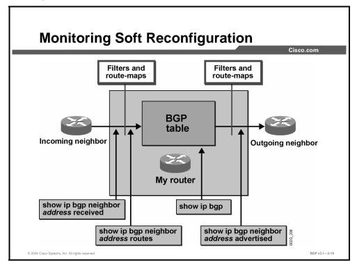
The **show ip bgp** command is used to display the local BGP table. You can check the entries that have been propagated to a specific neighbor with the **show ip bgp neighbor** *ip-address* **advertised** command. It displays the subset of the local BGP table that has passed the splithorizon check and all outgoing filters for the neighbor.
