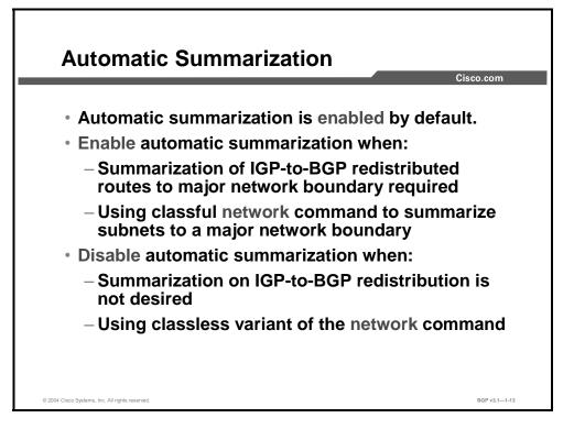
When a BGP router is configured to locally announce routes into BGP, the behavior of the **network** command varies depending on whether automatic summarization is enabled or disabled. When automatic summarization is enabled, BGP summarizes the locally originated BGP networks (network x.x.x.x) to their classful boundaries. Automatic summarization is enabled by default in BGP.
