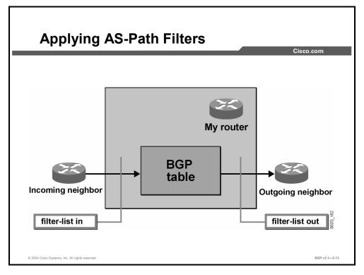
AS-path filters that are configured on a router select those routes that are allowed. Routes that are selected behave as follows:
