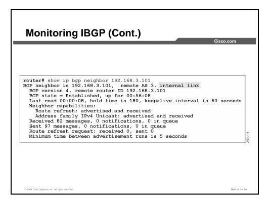
The **show ip bgp neighbors** command displays whether a router is running an IBGP (internal) or EBGP (external) session with a BGP neighbor. The indication is given by the "internal link" phrase (marked white in the second line of the figure).
