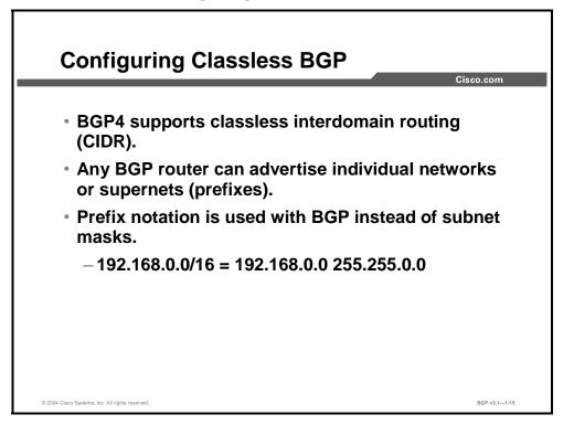
BGP4 is a classless protocol, meaning that its routing updates include IP address and the subnet mask. The combination of the IP address and the subnet mask is called an IP prefix. An IP prefix can be a subnet, a major network, or a supernet.
