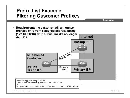
In this example, a multihomed customer has been assigned the address space 172.16.0.0/16. The customer may subnet this address space but may not announce smaller subnets than a subnet mask of 255.255.255.0. Larger subnets are accepted. If the customer has subnetted the network into smaller subnets, it must summarize the routing information about those subnets into at least /24 prefixes before announcing them.
