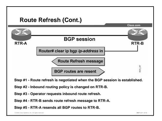
The capability to use the route refresh feature must be negotiated by the router when the BGP session is first established. The local router keeps a record that the capability is available with the neighbor. There is no need to keep a copy of the routing information that is received from the neighbor if it has the capability to refresh.
