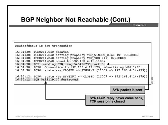
In the example here, the remote BGP router is not available. The sending router, therefore, never receives the reply to the SYN packet and aborts the TCP session in approximately 45 sec (changing the state from synsent to closed).
