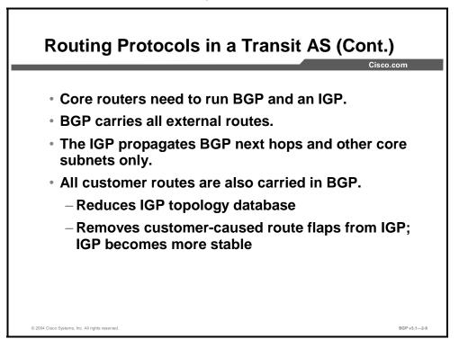
Both BGP and the configured IGP should be configured on all core routers inside the transit AS. The IGP should carry as little information as possible—ideally only the links within the core network, the loopback interfaces, and the external subnets that are used in EBGP sessions with neighboring autonomous systems. This information is enough to establish IBGP sessions and resolve next-hop addresses. The IGP will also work better if it carries less routing information.
