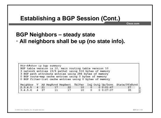
After the BGP sessions are in the Established state, routing information exchange can take place. The **show ip bgp summary** command output here indicates that a session is established by not displaying any information at all in the "State" column.
