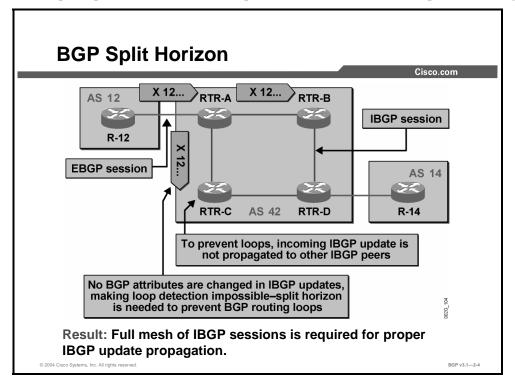
All routers within an AS must make routing decisions in a consistent way. They must have access to the same routing information with the same attributes in order to come to the same conclusion about which exit point of the AS to use. In other words, the BGP attributes should not be changed within the AS.
