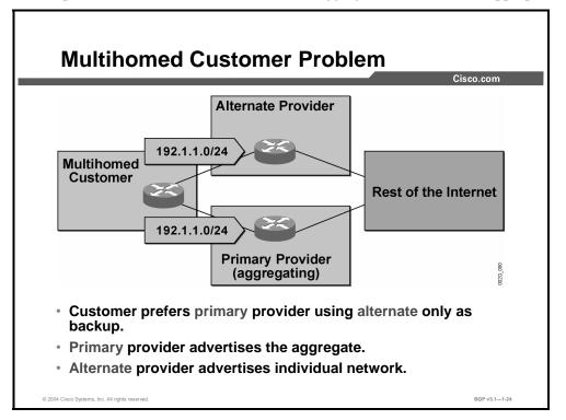
In this example, the primary provider is doing aggregation of 192.1.0.0/16 before sending it to the rest of the network. This situation means that the primary provider is also doing proxy aggregation for the route 192.1.1.0/24 that is advertised by the multihomed customer. The rest of the Internet will not see the route 192.1.1.0/24 via the primary provider.
