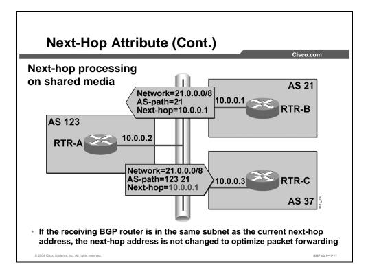
The next-hop processing changes if the BGP routers connect to a shared subnet. In the figure here, if RTR-A announces the network 21.0.0.0/8 to RTR-C with the BGP next-hop address set to RTR-A, the packets from AS 37 toward network 21.0.0.0/8 will have to cross the shared LAN twice. RTR-A thus sends the routing update toward RTR-C with the BGP next-hop address unchanged (still pointing toward RTR-B), allowing optimal data transfer across the shared LAN.
