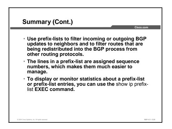
3-62 Configuring BGP on Cisco Routers (BGP) v3.1 Copyright © The PDF files and any printed representation for this material are the property of Cisco Systems, Inc., for the sole use by Cisco employees for personal study. The files or printed representations may not be used in commercial training, and may not be distributed for purposes other than individual self-study.
