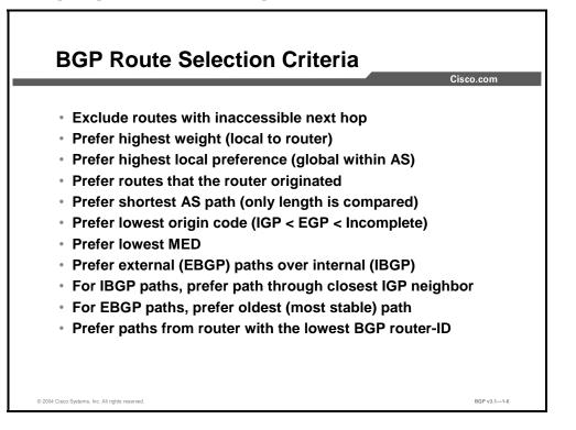
When a router has more than one alternative route to reach the same IP subnet (network and mask), the router has to select one of them as best in its default mode of operation. In order to make this selection, the router uses the BGP attributes that are attached to the different updates. The selection criteria are checked in the order that is indicated in the following steps. The first of the checks that indicates a difference is used, and no further testing is done.
