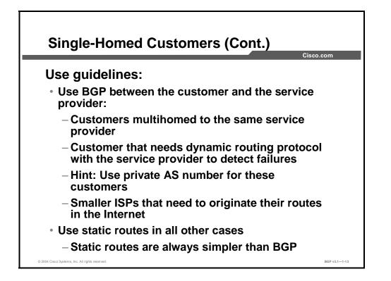
Under certain conditions, BGP must be configured between the customer and the service provider. For example, BGP is needed when customers are multihomed to the same service provider (that is, the customer networks have multiple links connecting them with the service provider network) and require dynamic routing protocol interaction with the service provider to detect link failures. Private AS numbers (AS numbers above 64512) are usually implemented in BGP configurations for these customers.
