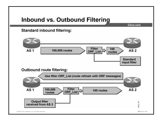
Outbound route filtering can limit the number of unwanted routing updates, which will reduce the amount of resources that are required for routing update generation and processing. This feature also reduces the amount of resources that are required to receive and discard routes that would otherwise be filtered out by the receiving router if the ORF feature was not available.
