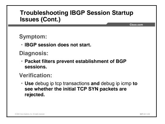
Packet filters can stop the BGP sessions. The path between the two BGP peer routers must be free from filters blocking the BGP traffic.
