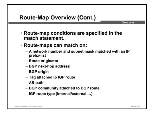
Each route-map statement can have several match clauses. Each match clause is given its own configuration line. The match clause refers to the tests to be made on the candidate route. Tests of the candidate route can be based on the following criteria:
