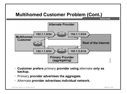
The rest of the Internet now sees overlapping routes. It sees 192.1.1.0/24 as reachable via the alternate provider and 192.1.0.0/16 as reachable via the primary provider. These two routes are treated as different routes. They are not compared with each other in a route selection process because they indicate different destinations. Because the router views them as different destinations, both routes will be injected into the routing table.
