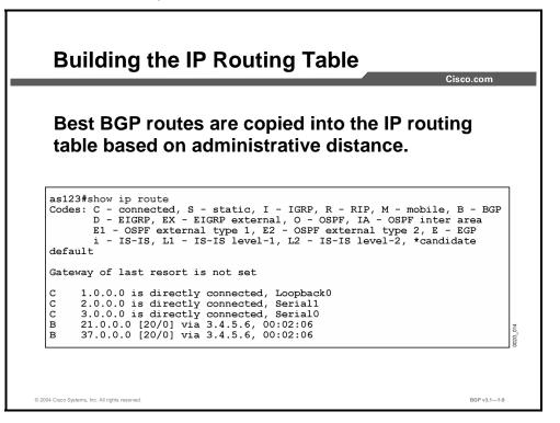
The route in the BGP table that BGP selects as the best is a candidate for installation in the IP forwarding, or routing, table.
