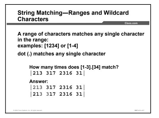
The pair of brackets "[" and "]" has a special meaning. They surround a set of characters of which any one matches. The set of characters is either expressed as the list of them (for example, "[1234]") or the sequence with the starting character, a hyphen, and the ending character (for example, "[1-4]"). Both examples match one single character, which must be any one in the set of the four characters "1", "2", "3", and "4".
