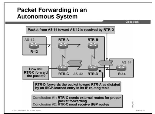
In this example, after AS 14 has received the routing information about reachable networks inside AS 12, IP packets can start to flow (in the figure, from AS 14 toward AS 12). R-14, the egress router in AS 14, forwards IP packets with destinations in AS 12 toward RTR-D, according to information received through EBGP.
