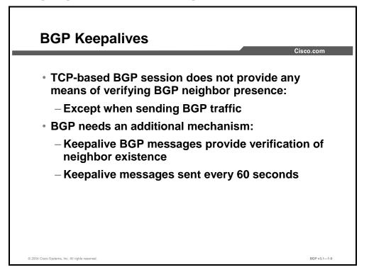
TCP-based BGP sessions do not provide any means of verifying the presence of a BGP neighbor. After BGP has established the TCP session, the only method of verifying neighbor presence is to actually send BGP traffic. BGP traffic is sent over the TCP session with acknowledgments (ACKs), and is therefore reliable. Successfully sending BGP traffic confirms the existence of a BGP neighbor.
