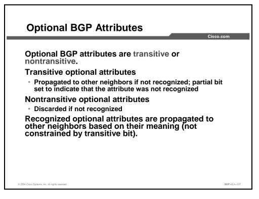
When a router receives an update that contains an optional attribute, the router checks to see if its implementation recognizes the particular attribute. If it does, then the router should know how to handle it and whether to propagate it or not.
