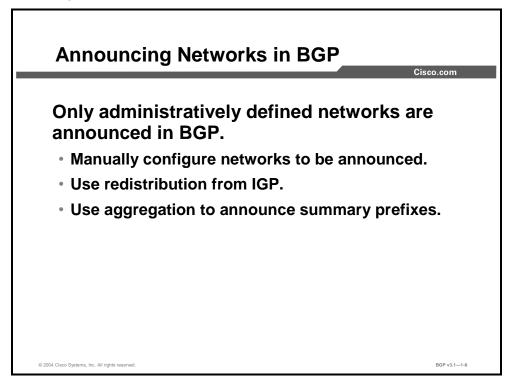
Before any local routing information can be injected by a router into its BGP table for advertising to other BGP routers, some basic configuration is required.
