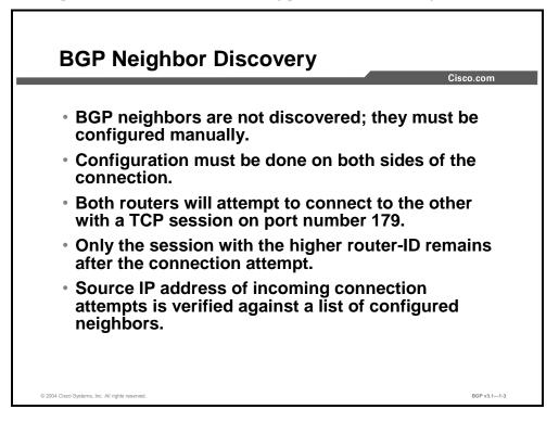
Unlike other routing protocols, BGP has no means of automatically detecting neighbors. The BGP protocol is carried in a TCP session, which must be opened from one router to the other. In order to do so, the router attempting to open the session must be manually configured with neighbor information indicating to which IP address to direct its connection attempts.
