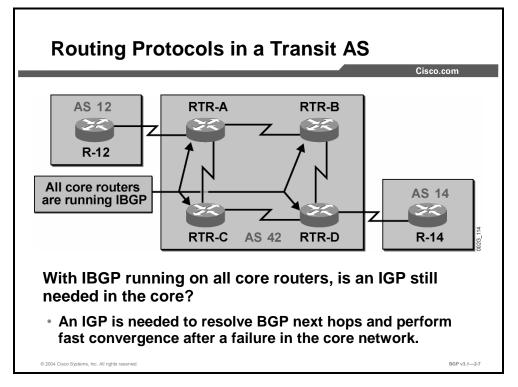
Some network designers base their network design on the wrong assumption that an internal routing protocol is not needed in a transit AS where all routers run BGP. However, the internal routing protocol is still needed inside an AS for two reasons:
