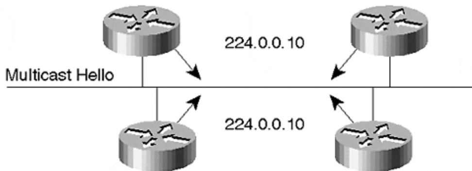
Figure 8-5. Hello Packets Sent to a Multicast Address for a Neighbor Relationship
