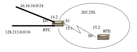
Suppose we added two static routes pointing to E0 on RTC: 16.16.16.0 255.255.255.0 (the /24 notation indicates a 24 bit mask starting from the far left) and 128.213.0.0 255.255.0.0. The following shows the different
