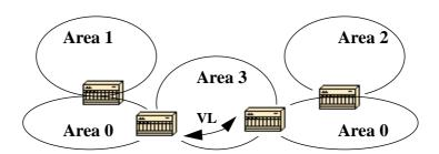
In the above diagram two area 0s are linked together via a virtual link. In case a common area does not exist, an additional area, such as area 3, could be created to become the transit area.
