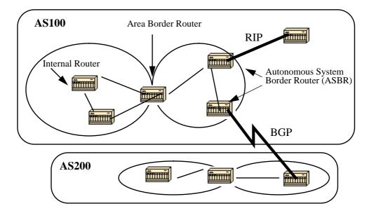
An area is interface specific. A router that has all of its interfaces within the same area is called an internal router (IR). A router that has interfaces in multiple areas is called an area border router (ABR). Routers that act as gateways (redistribution)between OSPF and other routing protocols (IGRP, EIGRP, IS-IS, RIP, BGP, Static) or other instances of the OSPF routing process are called autonomous system border routers (ASBR). Any router can be an ABR or an ASBR.
