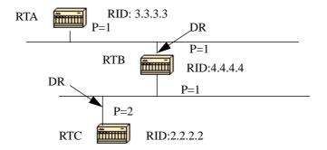
In the above diagram, RTA and RTB have the same interface priority but RTB has a higher RID. RTB would be DR on that segment. RTC has a higher priority than RTB. RTC is DR on that segment.
