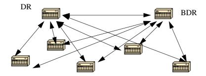
In the above diagram, all routers share a common multi-access segment. Due to the exchange of Hello packets, one router is elected DR and another is elected BDR. Each router on the segment (which already became a neighbor) will try to establish an adjacency with the DR and BDR.
