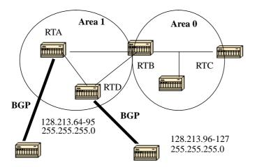
In the above diagram, RTA and RTD are injecting external routes into OSPF by redistribution. RTA is injecting subnets in the range 128.213.64-95 and RTD is injecting subnets in the range 128.213.96-127. In order to
