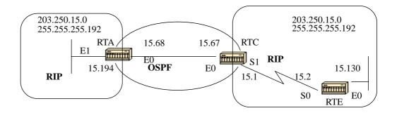
To illustrate, suppose RTA, RTC, and RTE are running RIP. RTC and RTA are also running OSPF. Both RTC and RTA are doing redistribution between RIP and OSPF. Let us assume that you do not want the RIP coming from RTE to be injected into the OSPF domain so you put a passive interface for RIP on E0 of RTC. However, you have allowed the RIP coming from RTA to be injected into OSPF. Here is the outcome (DO NOT USE THE FOLLOWING CONFIG-URATION):
