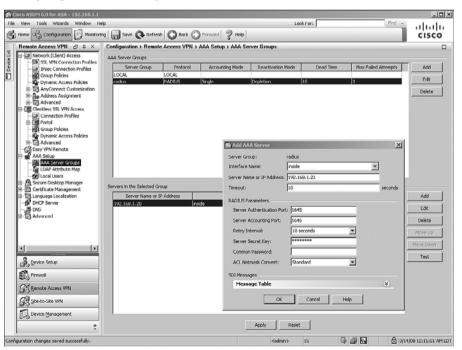
You can optionally modify the authentication and accounting port numbers if your RADIUS server does not use the default ports. The security appliance uses UDP ports 1645 and 1646 as defaults for authentication and accounting, respectively. Most of the RADIUS servers use ports 1812 and 1813 as authentication and accounting ports, respectively.
