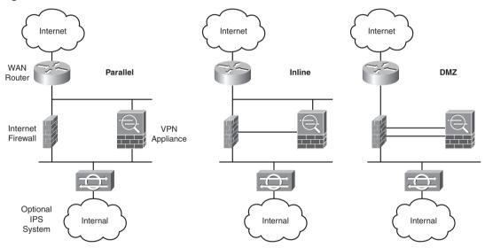
The device placement relationship between the SSL VPN appliance and Internet firewall is mainly based on the following two considerations:
