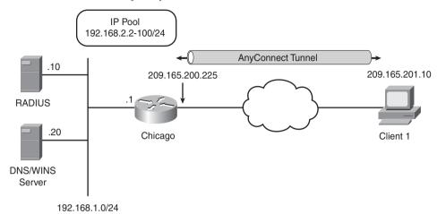
Figure 6-46 SecureMe's SSL VPN for AnyConnect Clients
