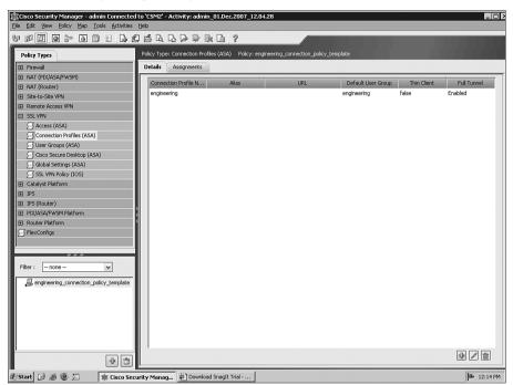
As shown in Figure 7-6, CSM handles ASAs and ISRs differently. For ASAs, the complete SSL VPN policy configuration is divided into five modules, each of which can be applied to ASAs separately. This gives you flexibility in terms of permutation of different modules into different policy sets. For ISRs, all aspects of the policy configuration are bundled together as one template.
