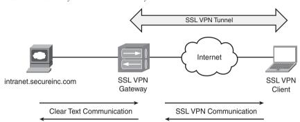
Figure 1-4 SSL VPN Gateway and Connection Proxy
