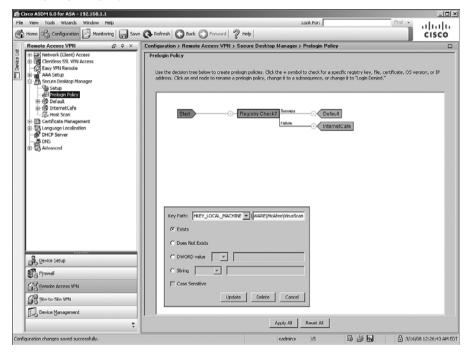
The workstations that have the registry setting are further accessed for additional checks. In Figure 5-48, workstations are checked for their IP addresses. If they are in the 192.168.1.0/24 subnet, they are identified as OfficeCorpOwned workstations. If they are not, they are identified as HomeCorpOwned workstations.
