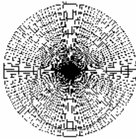
E-Plane Pattern - Upper Polarization 40 dB Gain Pattern (dBi)
