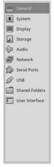
**General:** General Setting defines the virtual machine's name and operating system type. You will enable the clipboard on the Advanced tab to copy and paste text, files, and directories between the host and guest systems.
