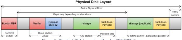
Figure 5: Physical Disk Layout written by DEBUGFILE.sys
