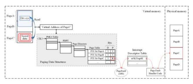
Figure 3 Log and manage access to memory pages by setting corresponding page table entry as non-present and replacing the page fault handler
