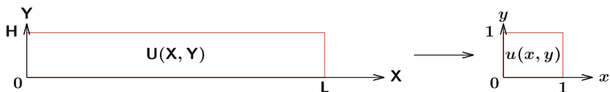
Fig. 8.1 The domain for problem (8.10), a slender rectangle in dimensional coordinates ( Left ) and the rescaled dimensionless domain ( Right )
